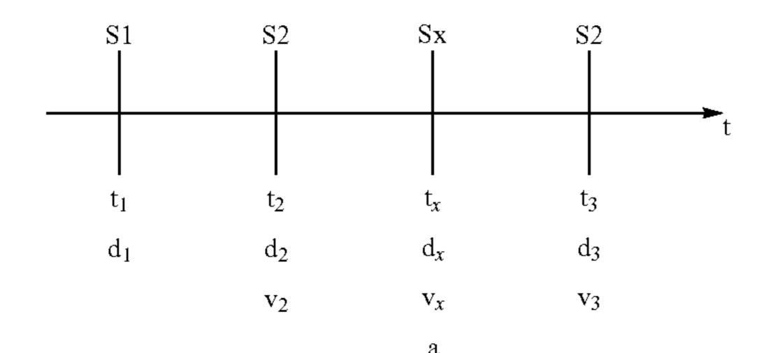
Using the change in position of the runner 12 between S1 and S2, the velocity of the runner 12 at S2  $(v_2)$  can be calculated. For example:
