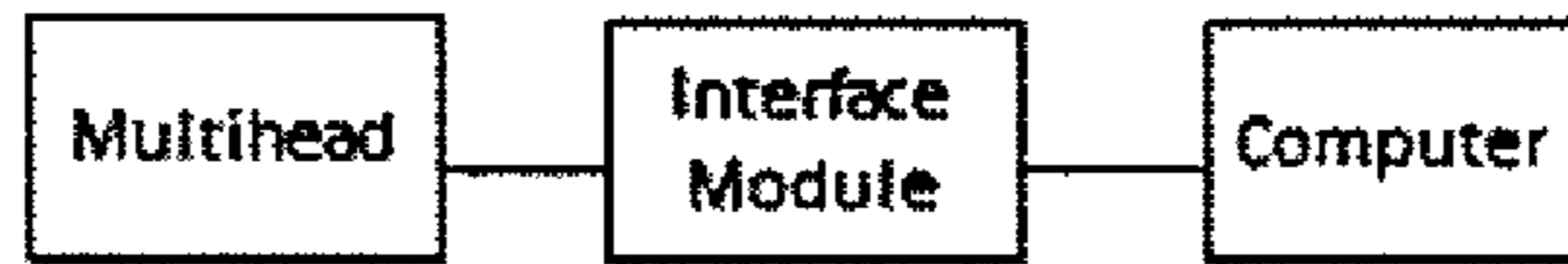
Figure 1b The Basic Gamma Camera System with several multiheads
