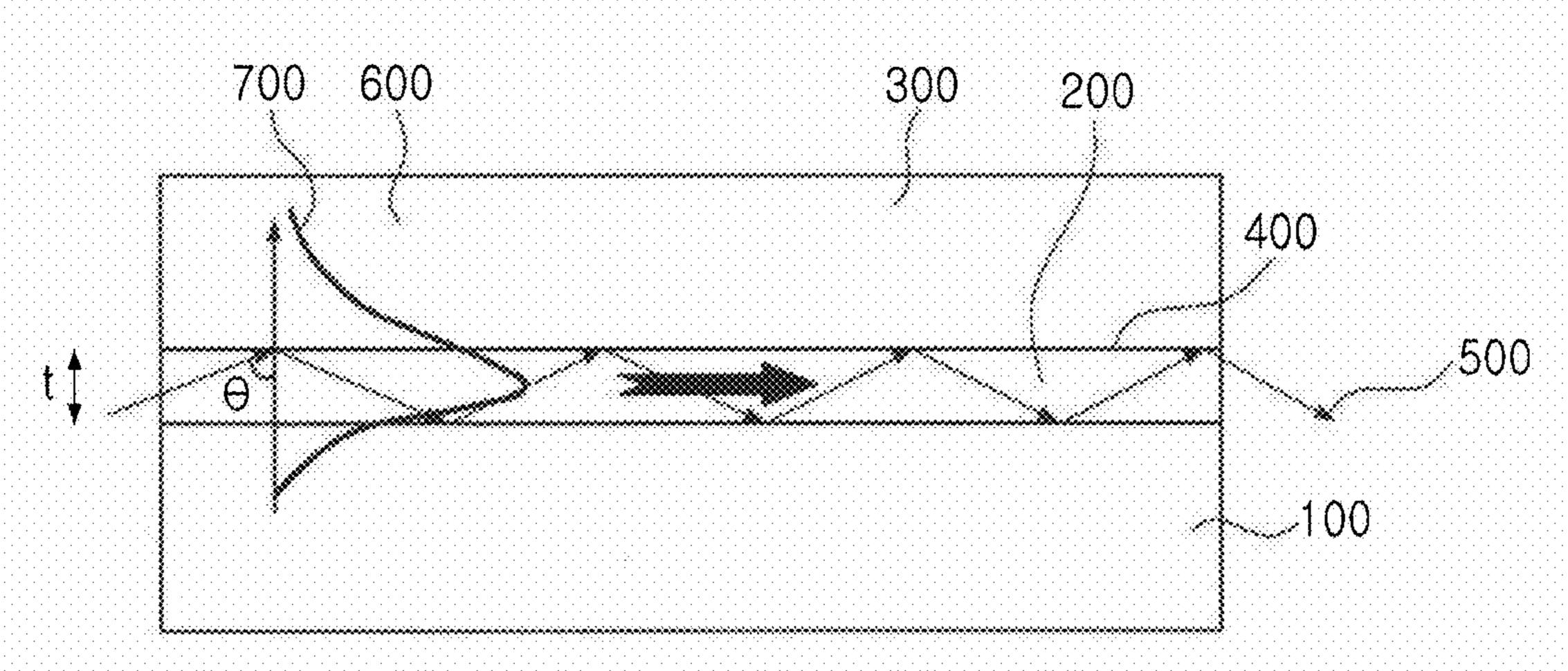
N (# of total internal reflection) = L / (2t tan  $\Theta$ ) (Example) L~5mm, t ~1µm, 0~40°  $\rightarrow$  N~3000 !!!
