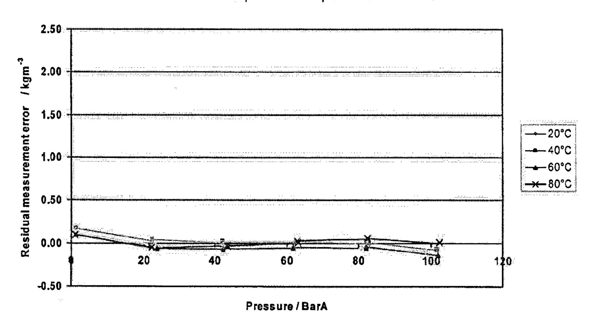
Figure 7  $\text{New performace with } K_{pt} \text{ on a fluid of base density } 914.0 \text{ kgm}^{-3}$  at combined temperature and pressure conditions
