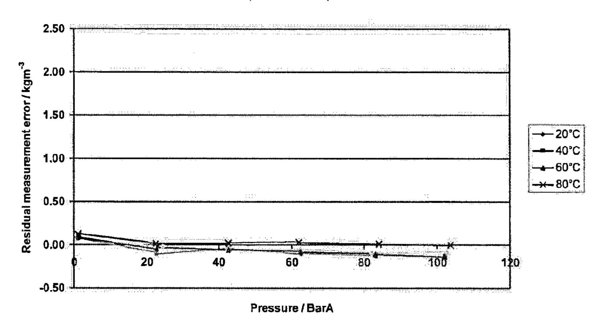
Figure 6 New performace with  $K_{22}$  and  $K_{23}$  on a fluid of base density 914.0 kgm<sup>-3</sup> at combined temperature and pressure conditions
