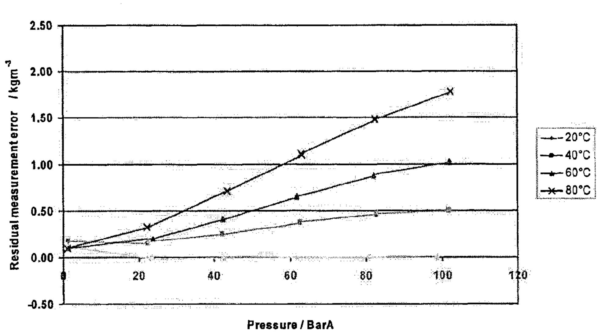
Figure 5 New performace with  $K_{22}$  and  $K_{23}$  on a fluid of base density 826.8 kgm<sup>-3</sup> at combined temperature and pressure conditions
