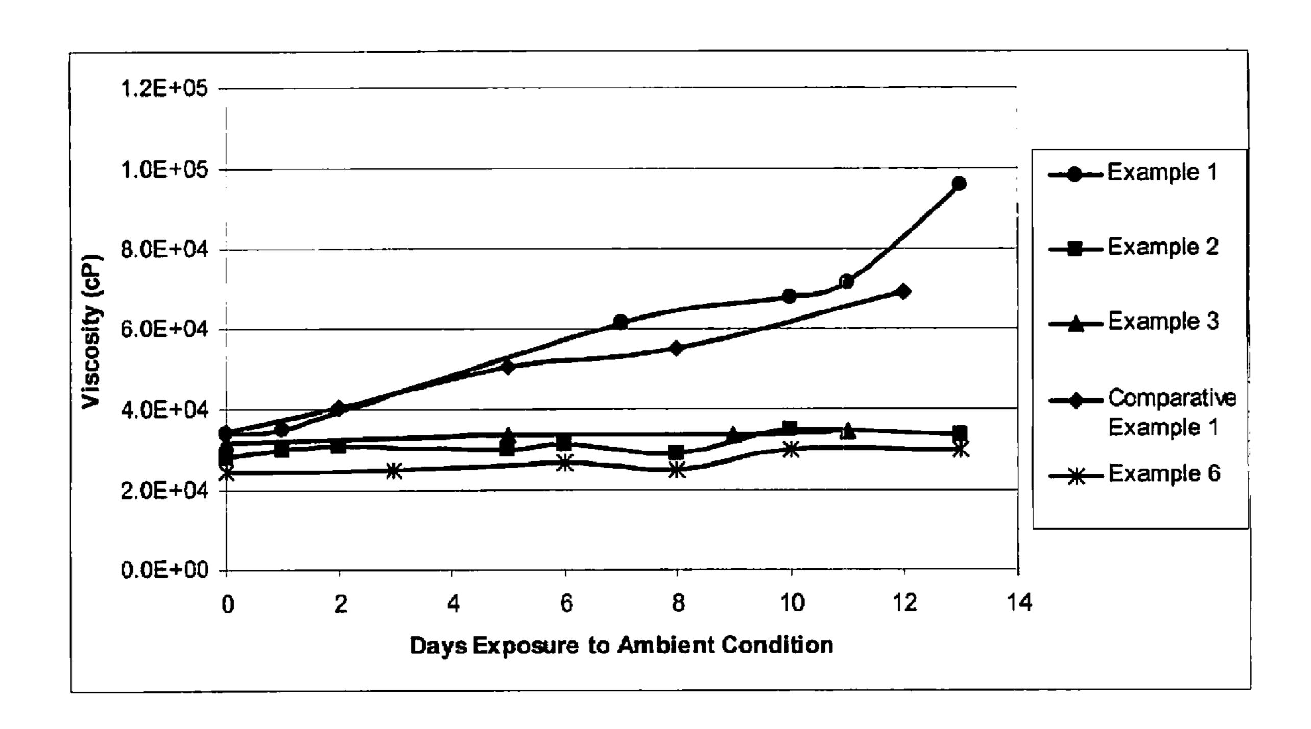
Viscosity of the Silylated Polyurethane Composition Exposure to Atmospheric Moisture at 23°C and 1 Atmosphere Pressure.
