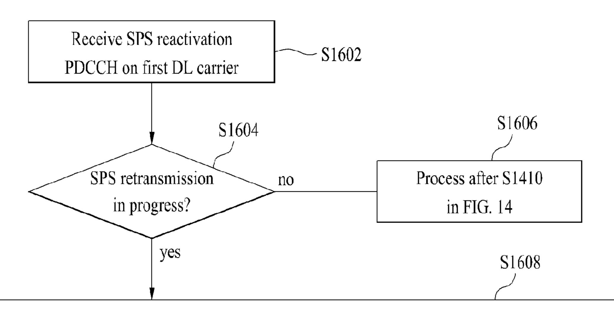
Option 1: SPS reactivation PDCCH is applied to DL/UL CC on which SPS retransmission is in progress irrespective of a presence or non-presence of CI information.
