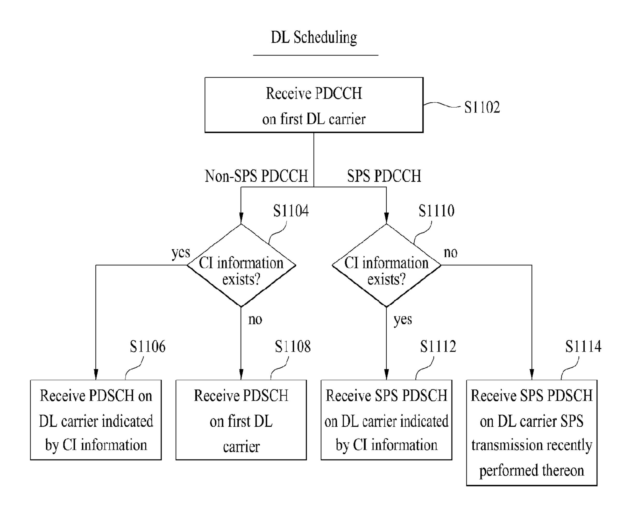
Note: In case of UL scheduling, PUSCH is transmitted on UL carrier indicated by CI information [S1106] or UL carrier linked with first DL carrier [S1108].
