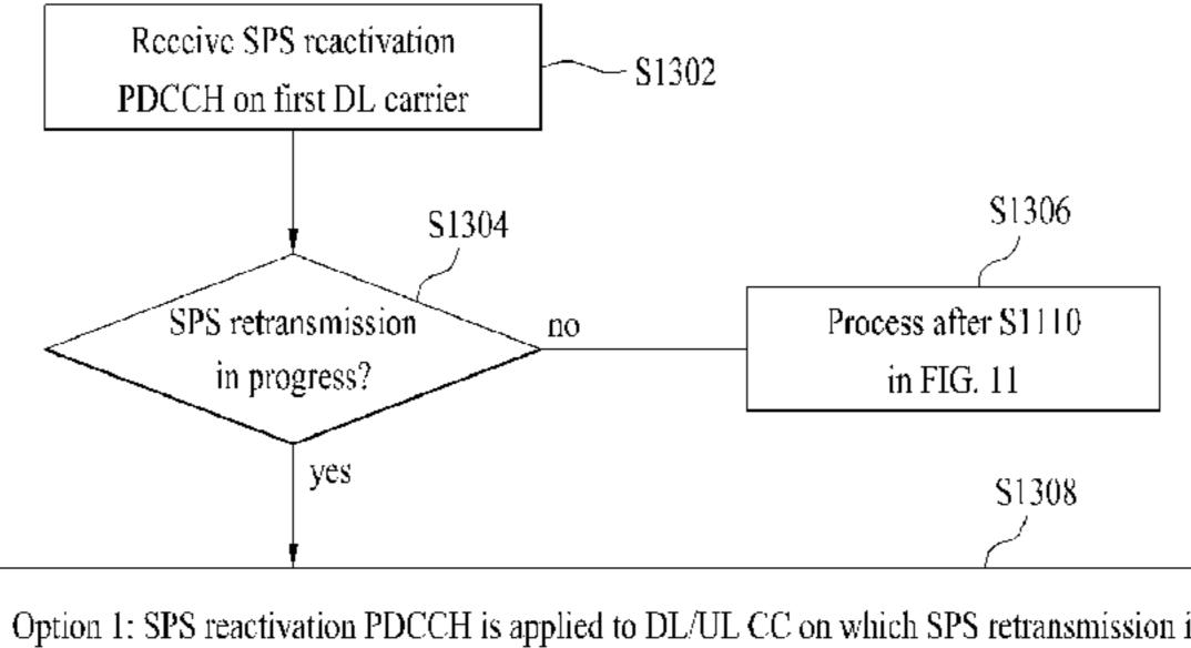
Option 1: SPS reactivation PDCCH is applied to DL/UL CC on which SPS retransmission is in progress irrespective of a presence or non-presence of CI information.
