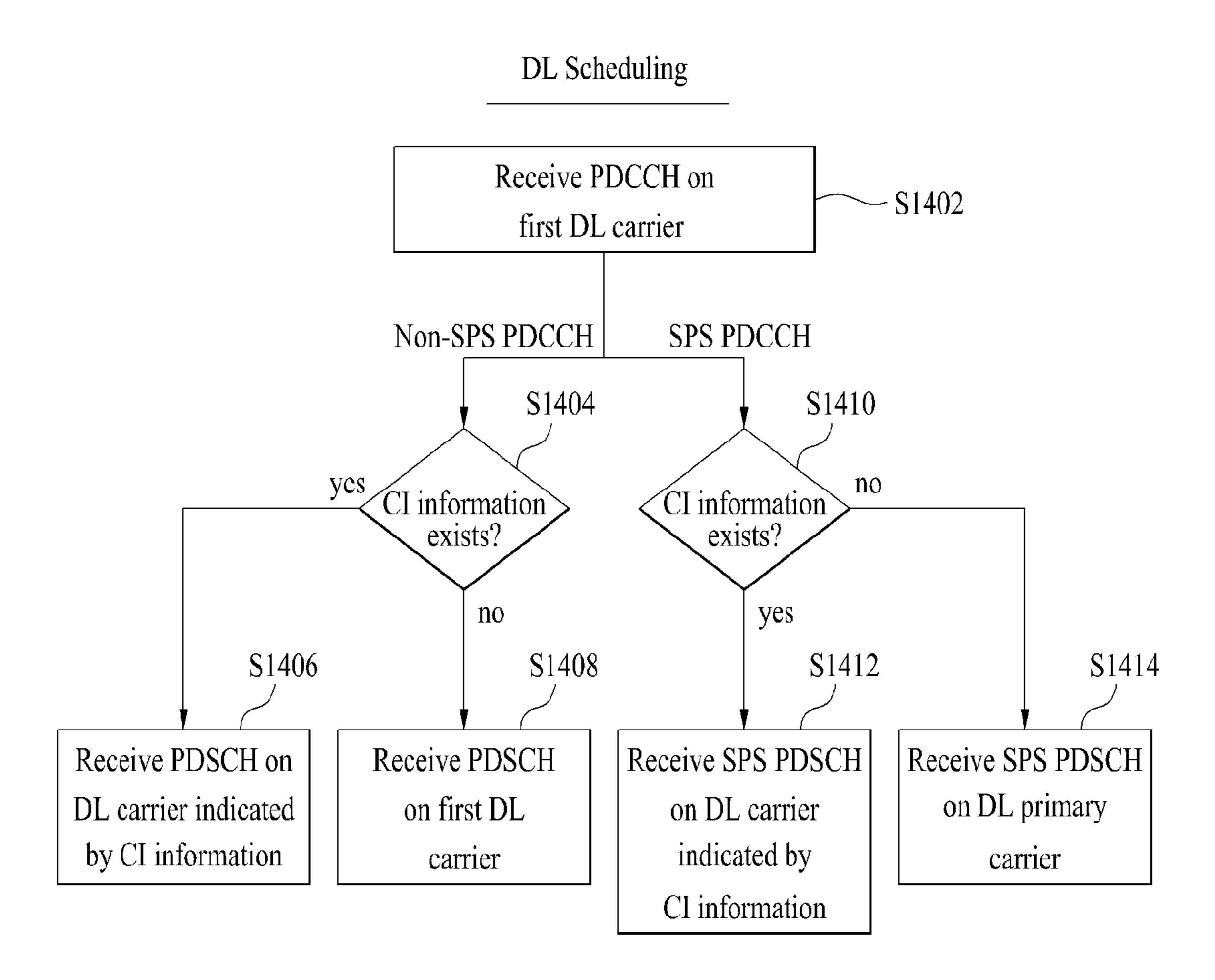
Note: In case of UL scheduling, PUSCH is transmitted on UL carrier indicated by CI information [S1406] or UL carrier linked with first DL carrier [S1408].
