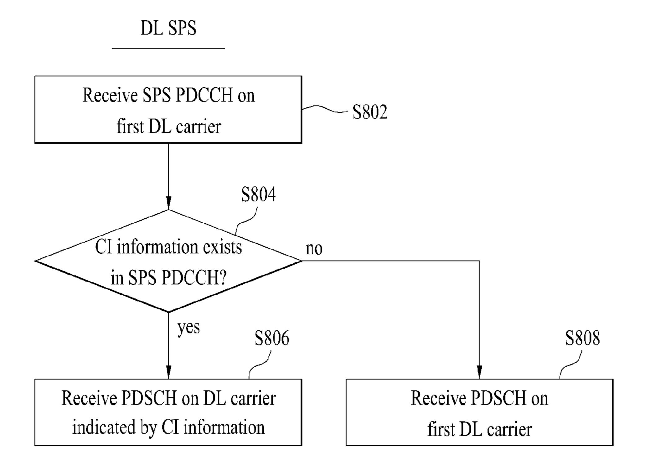
Note: In case of UL SPS, PUSCH is transmitted on UL carrier indicated by CI information [S806] or UL carrier linked with first DL carrier [S808].
