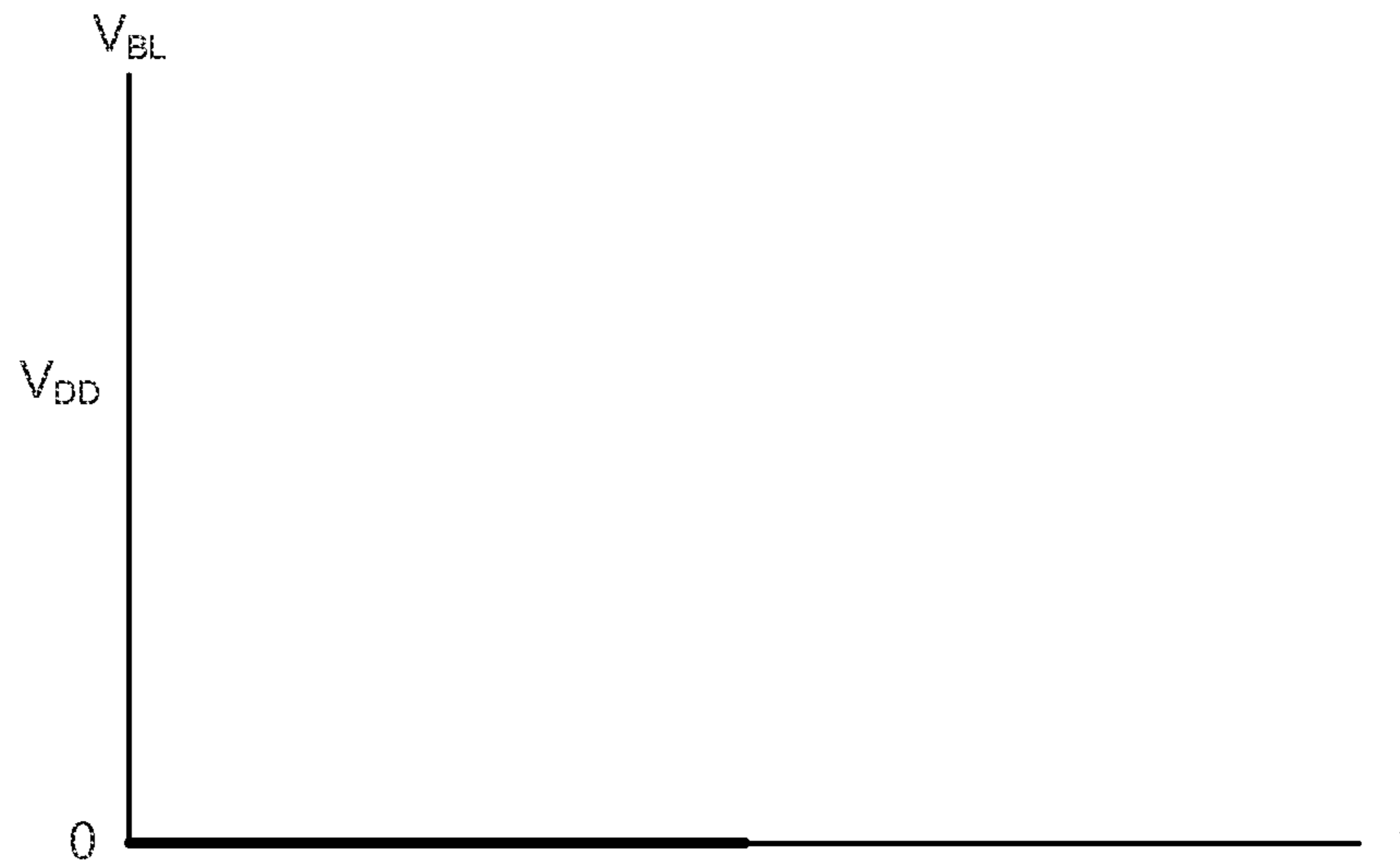
Setting the Bit Line to a program-enabled voltage
