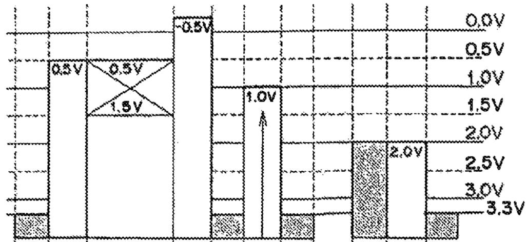
FIG. 5A  $t_3 < t < t_4$  TRANSFER OF SIGNAL CHARGE FROM PD TO FD
