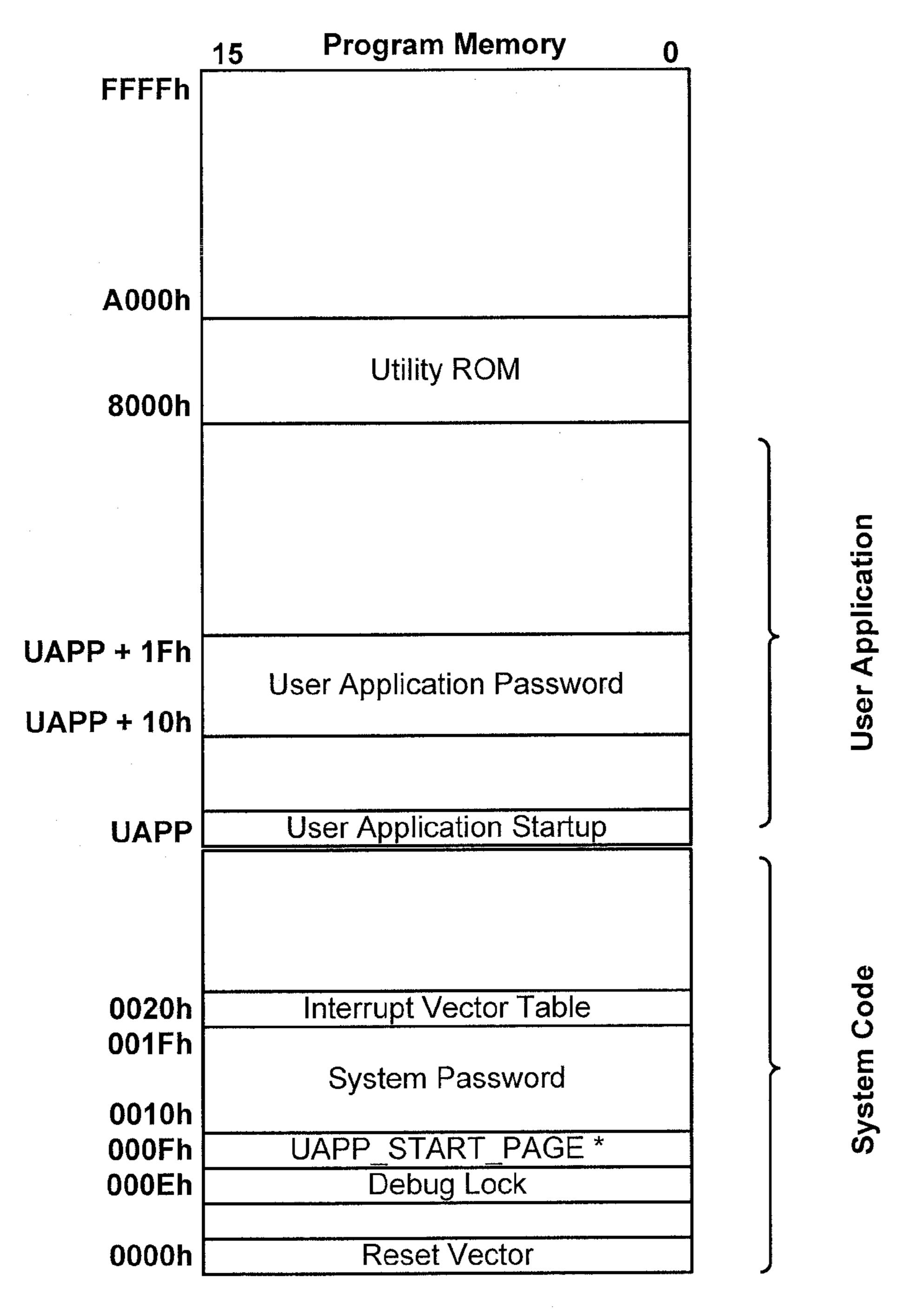
\* The Most Significatn Bit of UAPP\_START\_PAGE should be set to '1' for proper UROM JTAG loader context
