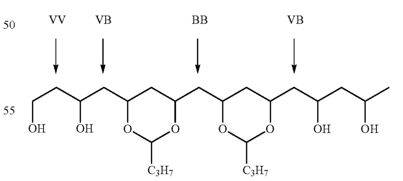
The OH blockiness of the polyvinyl acetals according to the invention is calculated from the quotient VV/(VB+BB) and can be ascertained by <sup>13</sup>C-NMR measurements, as illustrated hereinafter.
