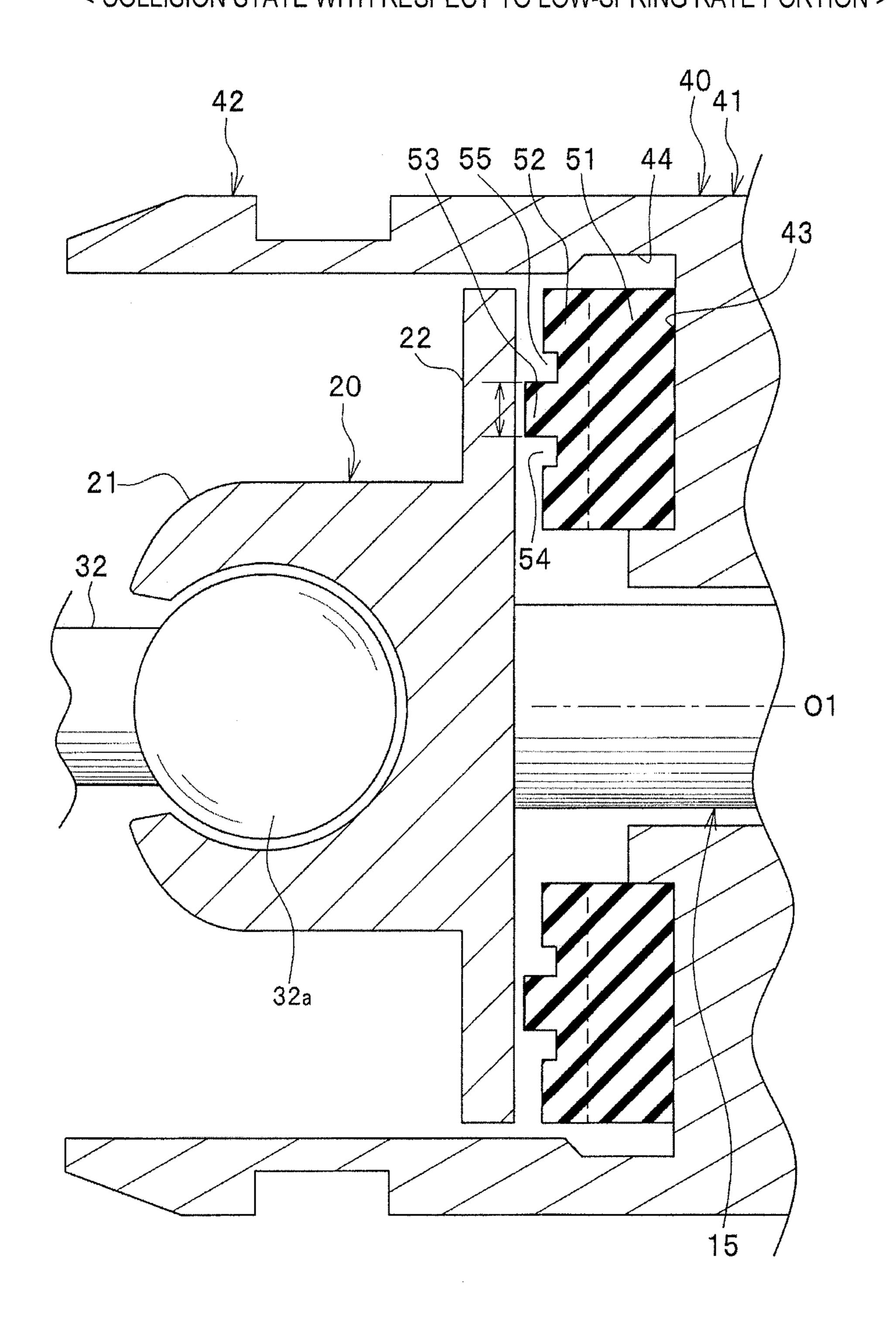
FIG. 5 < COLLISION STATE WITH RESPECT TO HIGH-SPRING RATE PORTION >
