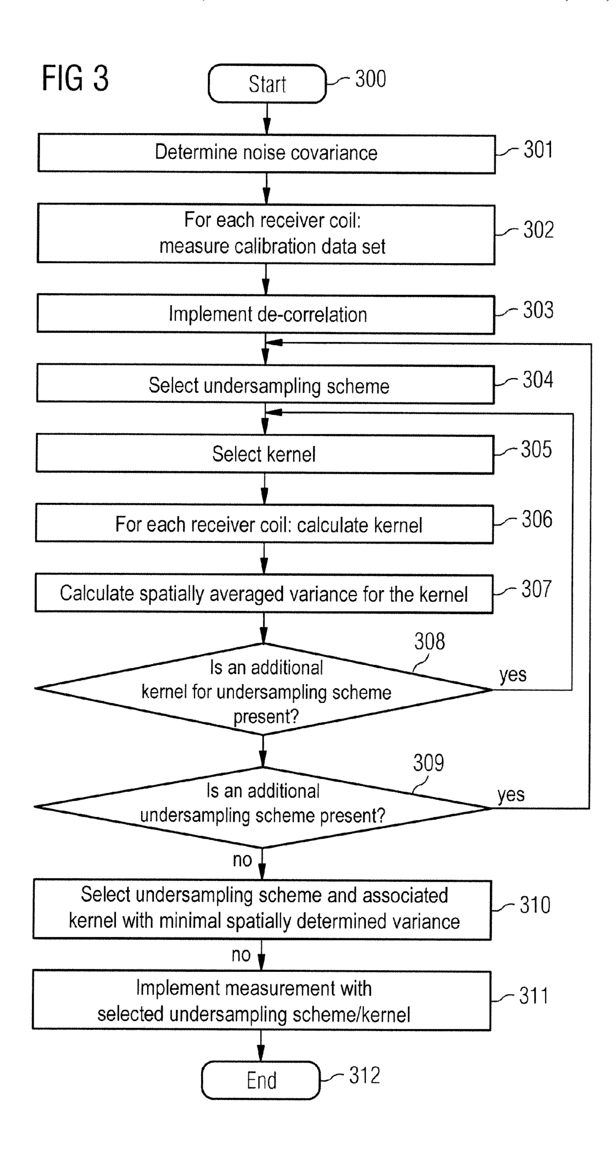
METHOD TO SELECT AN UNDERSAMPLING SCHEME FOR MAGNETIC RESONANCE IMAGING, AND MAGNETIC RESONANCE IMAGING METHOD AND SYSTEM USING SUCH A SELECTED UNDERSAMPLING SCHEME
