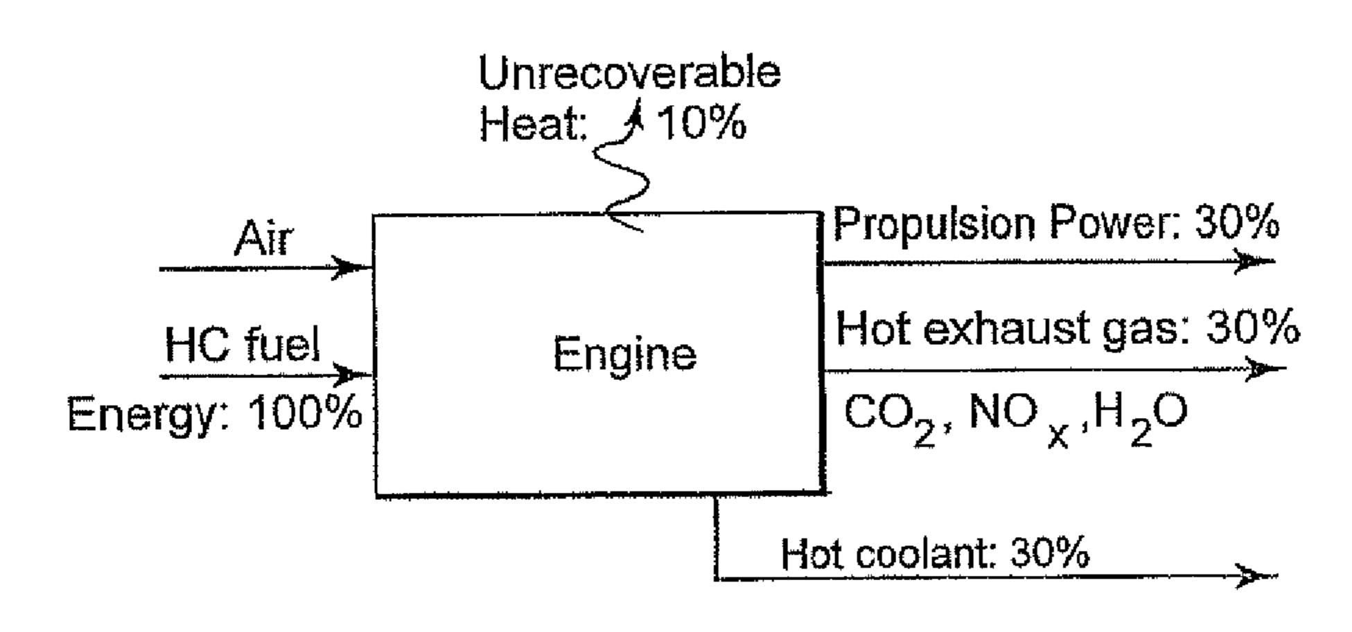
>Heat for regeneration of absorbent >Heat to power for compression or liquefaction of CO capture and: Hot exhaust gas: 30% Propulsion Power: 30%  $CO_2$ ,  $NO_x$ ,  $H_2O$ Hot coolant: 30% Unrecoverable Heats 10% Engine Energy: 100%
