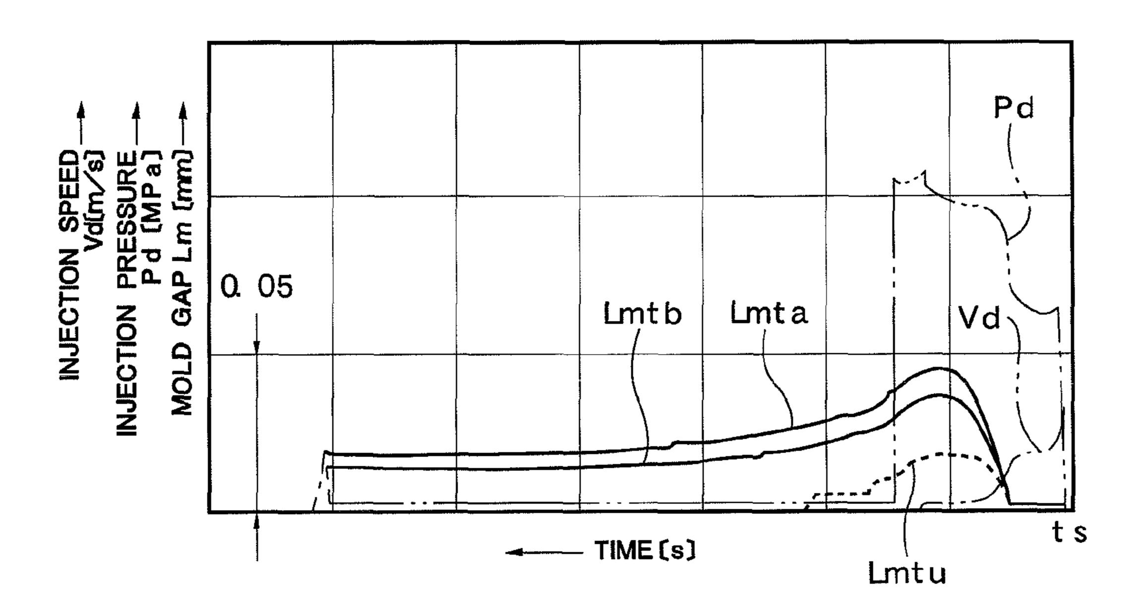
Lmta:MOLD POSITION 0. 8 (mm), CLAMPING FORCE 30 (%), NON-LOCK-UP STATE Lmtb:MOLD POSITION 0. 5 (mm), CLAMPING FORCE 30 (%), NON-LOCK-UP STATE Lmtu: MOLD POSITION 0 (mm), CLAMPING FORCE 30 (%), LOCK-UP STATE
