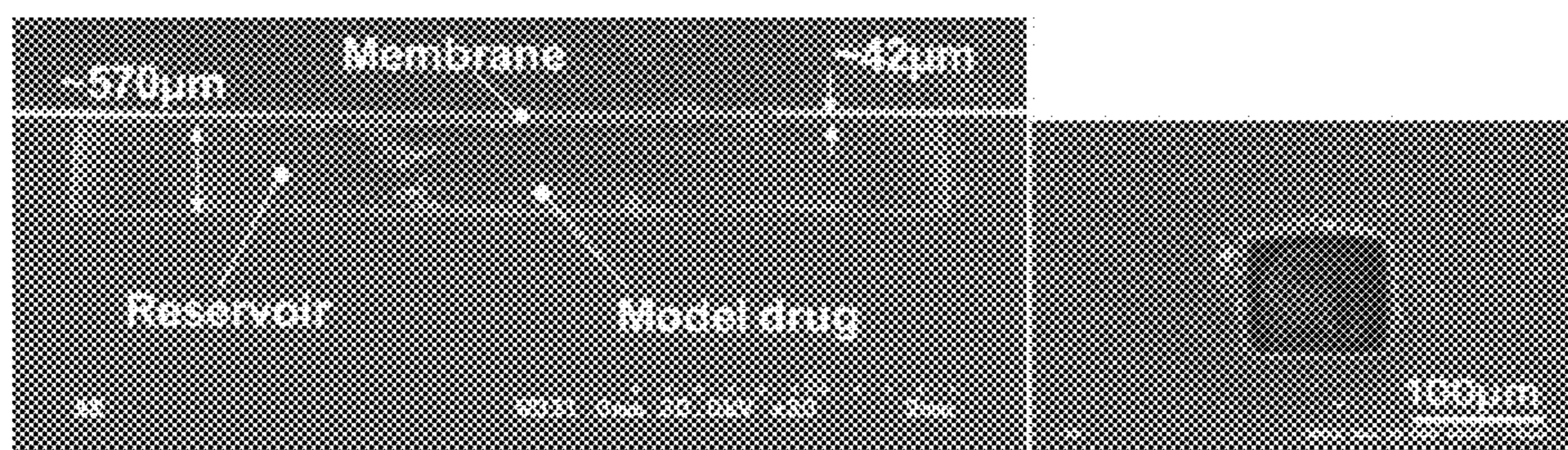
(a) Cross-section of a fabricated device showing free-standing magnetic membrane with residues of a model drug inside the reservoir; (b) Laser-drilled apertures in the magnetic membranes ablated using UV laser with 325 nm wavelength.
