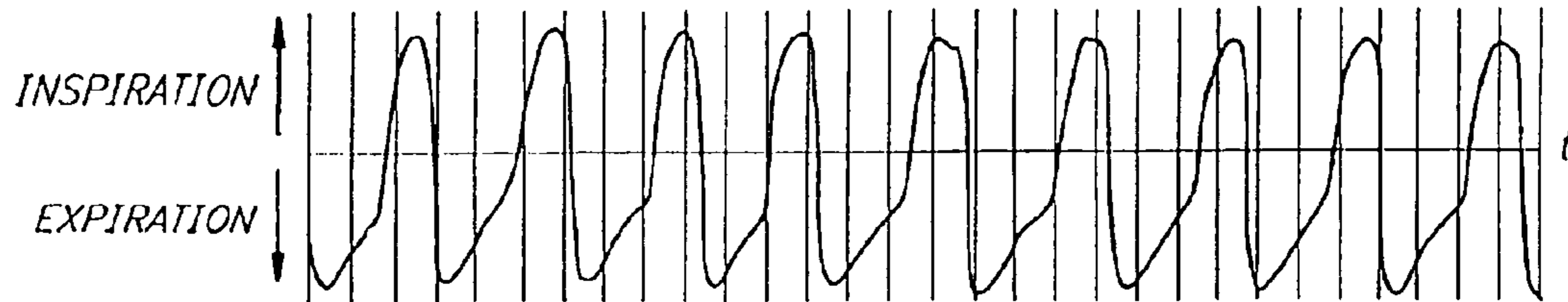
FIG. 1 AIRFLOW TO AND FROM CPAP GENERATOR
