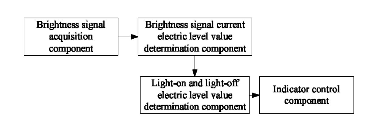
the brightness of a working environment of a terminal device is detected in real time to acquire a brightness signal of the working environment of the terminal device
