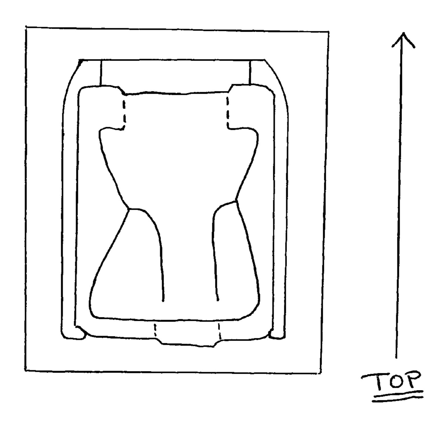
Side view; paper filter lying flat exposing acordian suspension and open side fillable top
