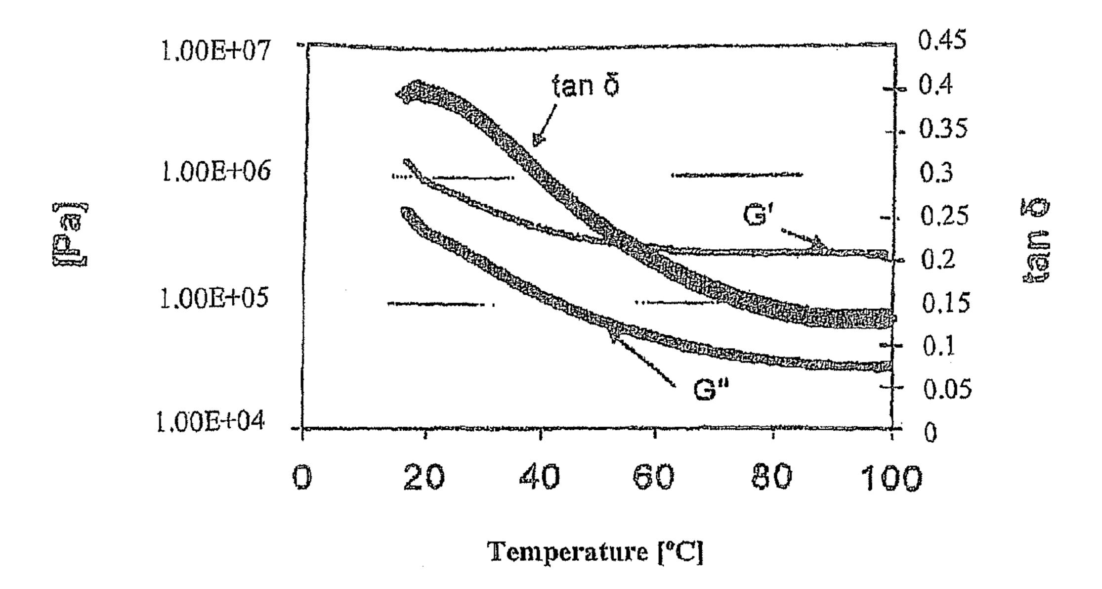
Storage modulus and loss modulus as well as loss factor  $\tan \delta$  of the viscoelastic polymer which is obtained by reacting the prepolymers with water in accordance with Example 4.
