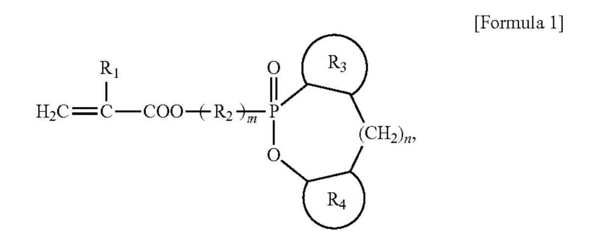
wherein  $R_1$  is hydrogen or methyl;  $R_2$  is a substituted or unsubstituted  $C_1$  to  $C_{20}$  hydrocarbon group;  $R_3$  and  $R_4$  are the same or different and are each independently a substituted or unsubstituted  $C_6$  to  $C_{20}$  cyclic hydrocarbon group; m is an integer from 1 to 10; and n is an integer from 0 to 5.
