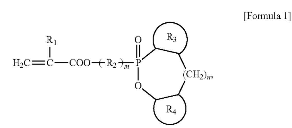
2. The thermoplastic copolymer according to claim 1, wherein the phosphorus (meth)acrylic monomer is present in 40 an amount of about 1 wt % to about 70 wt %, and the monomers comprising the aromatic vinyl monomer and the vinyl cyanide monomer are present in an amount of about 30 wt % to about 99 wt %.
