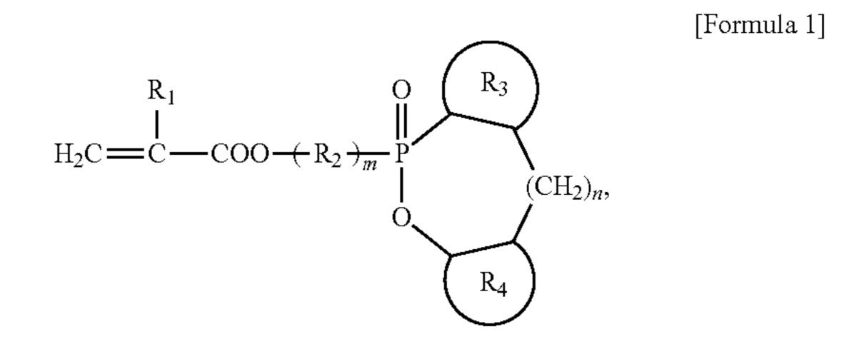
wherein  $R_1$  is hydrogen or methyl;  $R_2$  is a substituted or unsubstituted  $C_1$  to  $C_{20}$  hydrocarbon group;  $R_3$  and  $R_4$  are each independently a substituted or unsubstituted  $C_6$  to  $C_{20}$  cyclic hydrocarbon group; m is an integer from 1 to 10; and n is an integer from 0 to 5.
