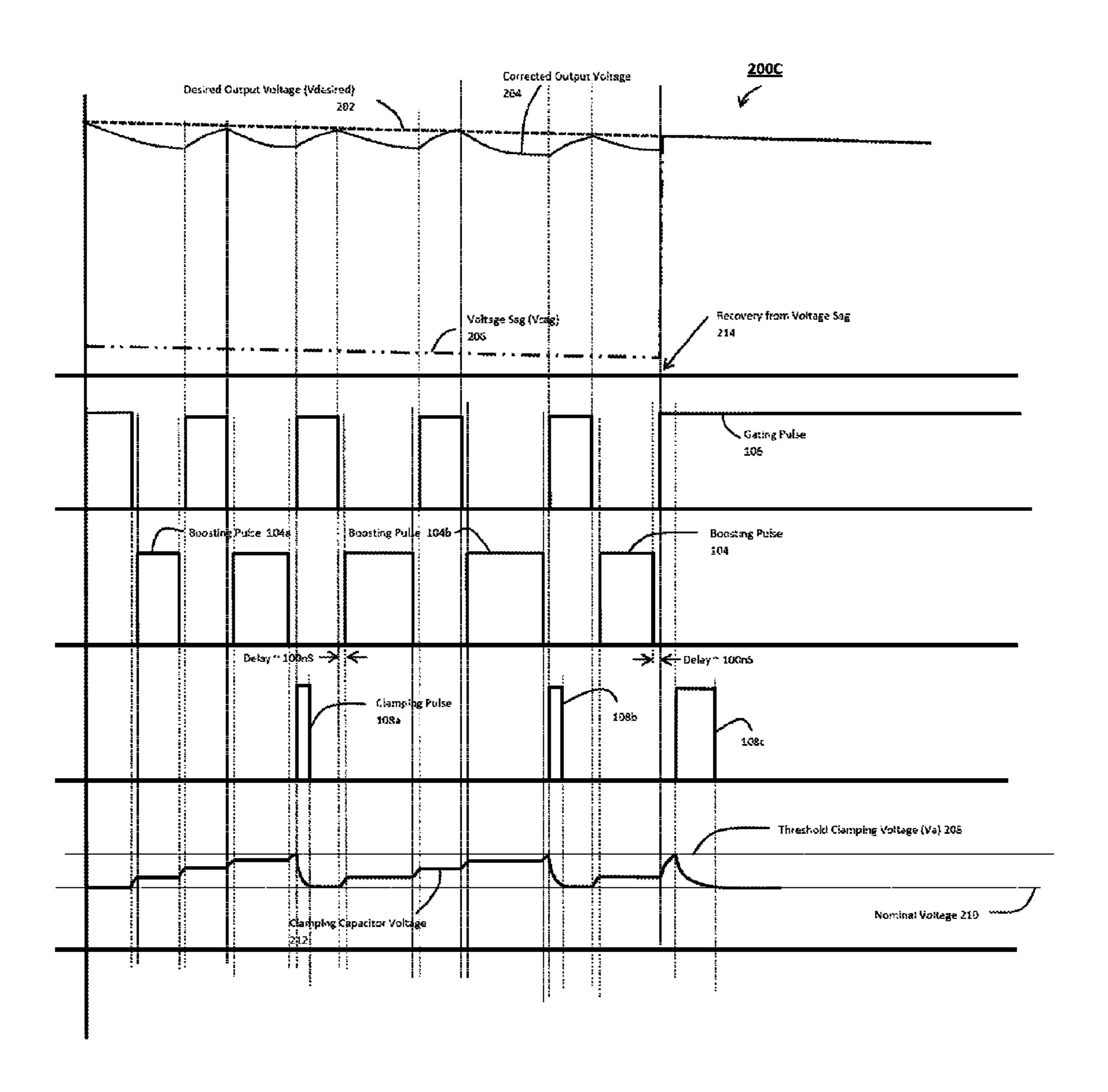
FIG 2C. EXEMPLARY VOLTAGE WAVEFORMS, BOOSTING PULSES, GATING PULSES, AND CLAMPING PULSES DURING SAG RECOVERY
