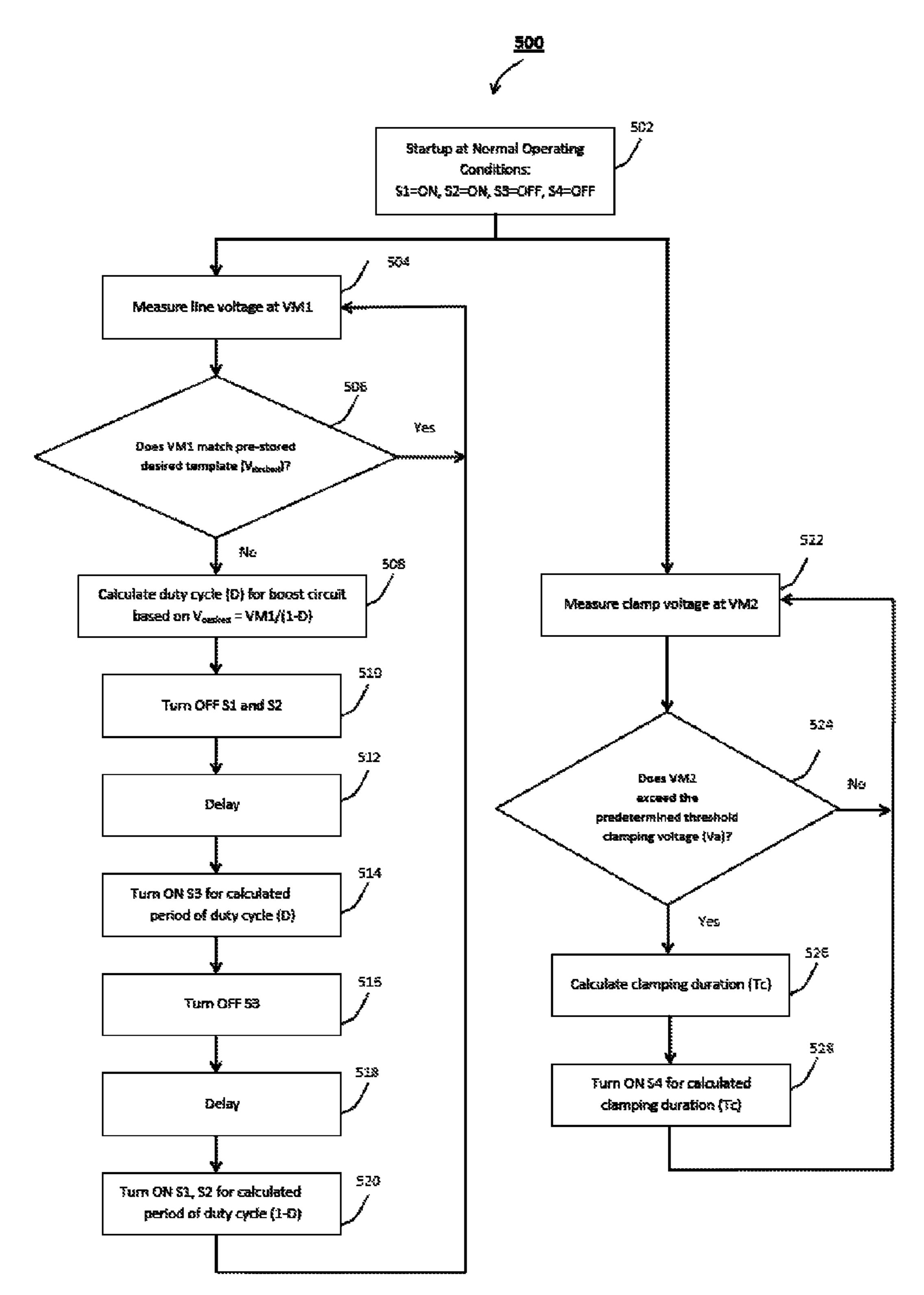
FIG 5. EXEMPLARY CONTROL CIRCUIT PROCESS
