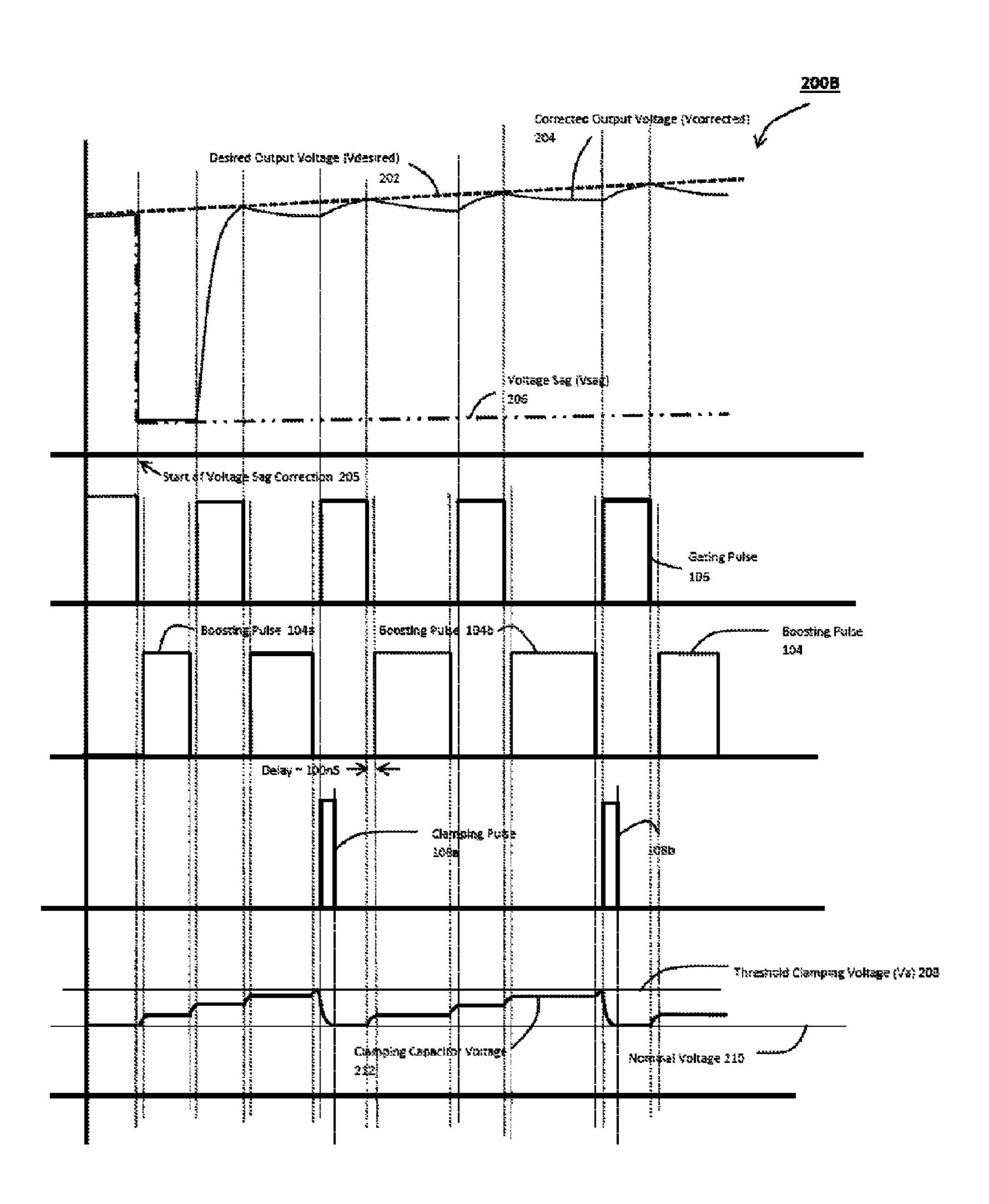
FIG 28. EXEMPLARY VOLTAGE WAVEFORMS, BOOSTING PULSES, GATING PULSES, AND CLAMPING PULSES DURING SAG CORRECTION
