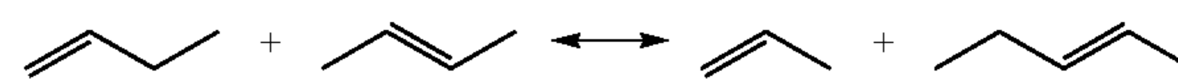
Heavies Formation During Metathesis in Presence of Iso-Butene
