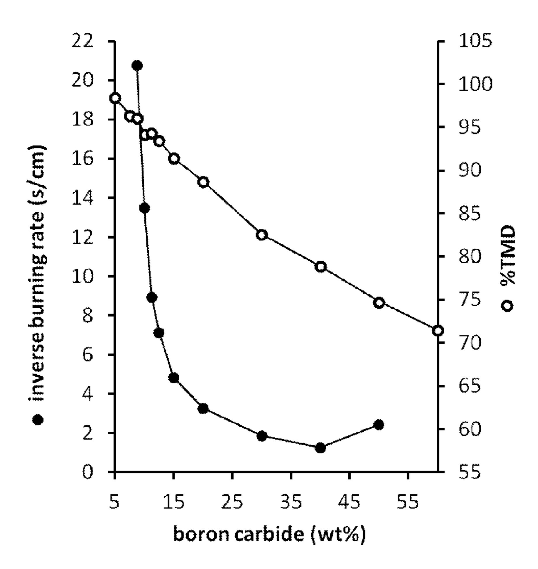
**Figure 1.** Inverse burning rates (s/cm, closed circles) and %TMD (open circles) for x/(90-x)/10 mixtures of B<sub>4</sub>C/NaIO<sub>4</sub>/PTFE.
