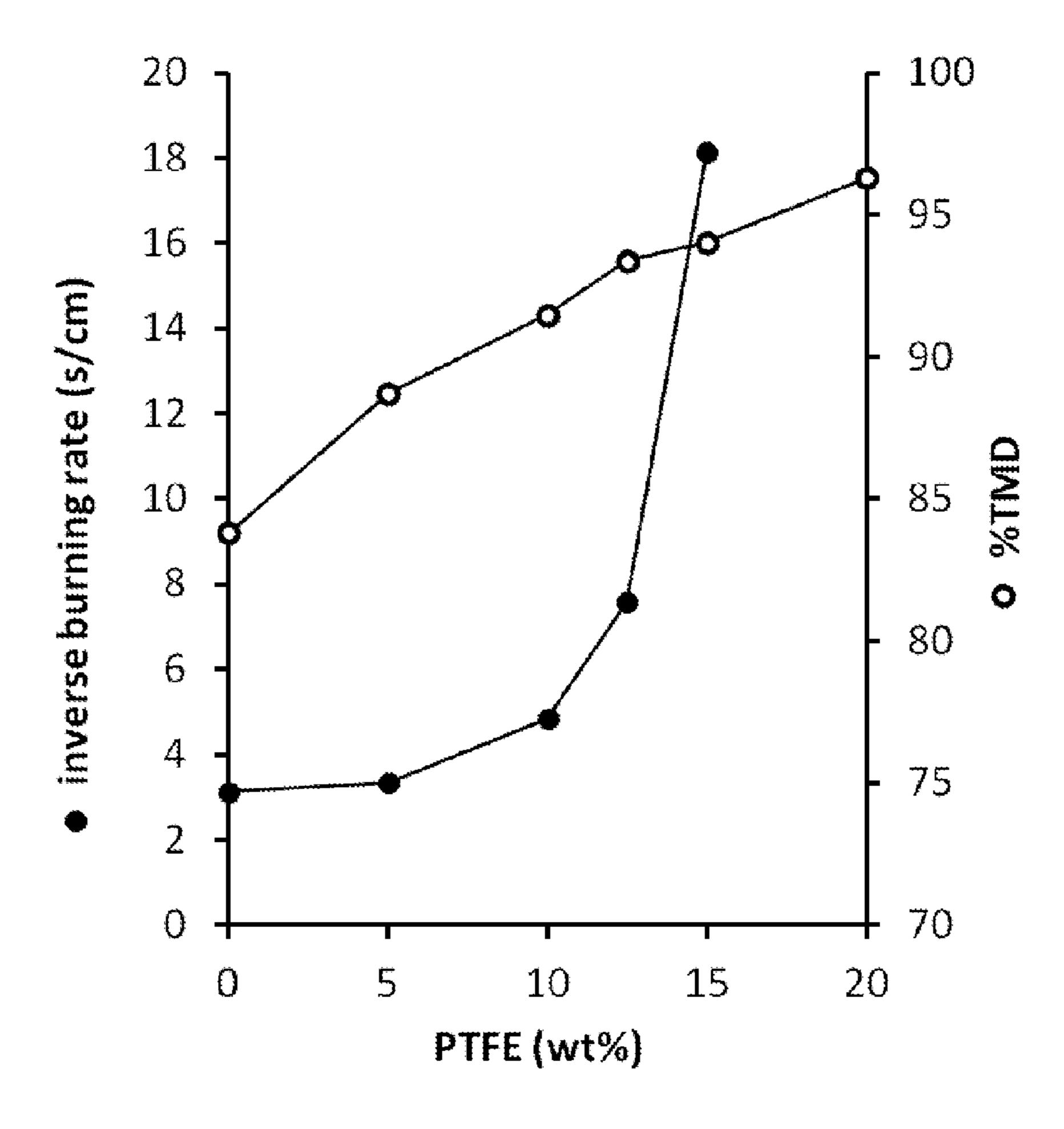
**Figure 2.** Inverse burning rates (s/cm, closed circles) and %TMD (open circles) for 15/(85-x)/x mixtures of B<sub>4</sub>C/NaIO<sub>4</sub>/PTFE.
