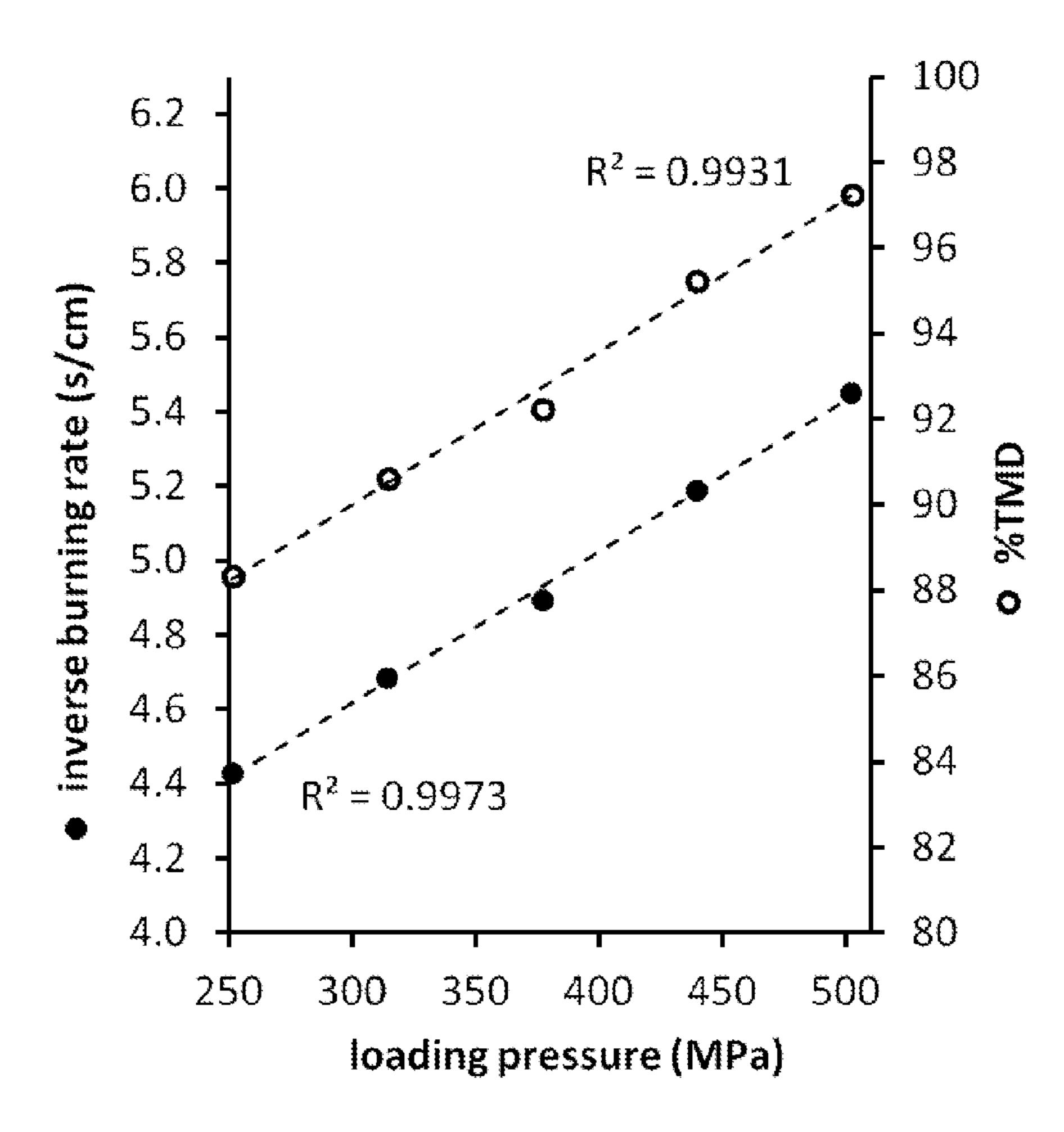
**Figure 3.** Inverse burning rate (s/cm, closed circles) and %TMD (open circles) as functions of loading pressure. Data is shown for a 15/75/10 mixture of  $B_4C/NalO_4/PTFE$ .
