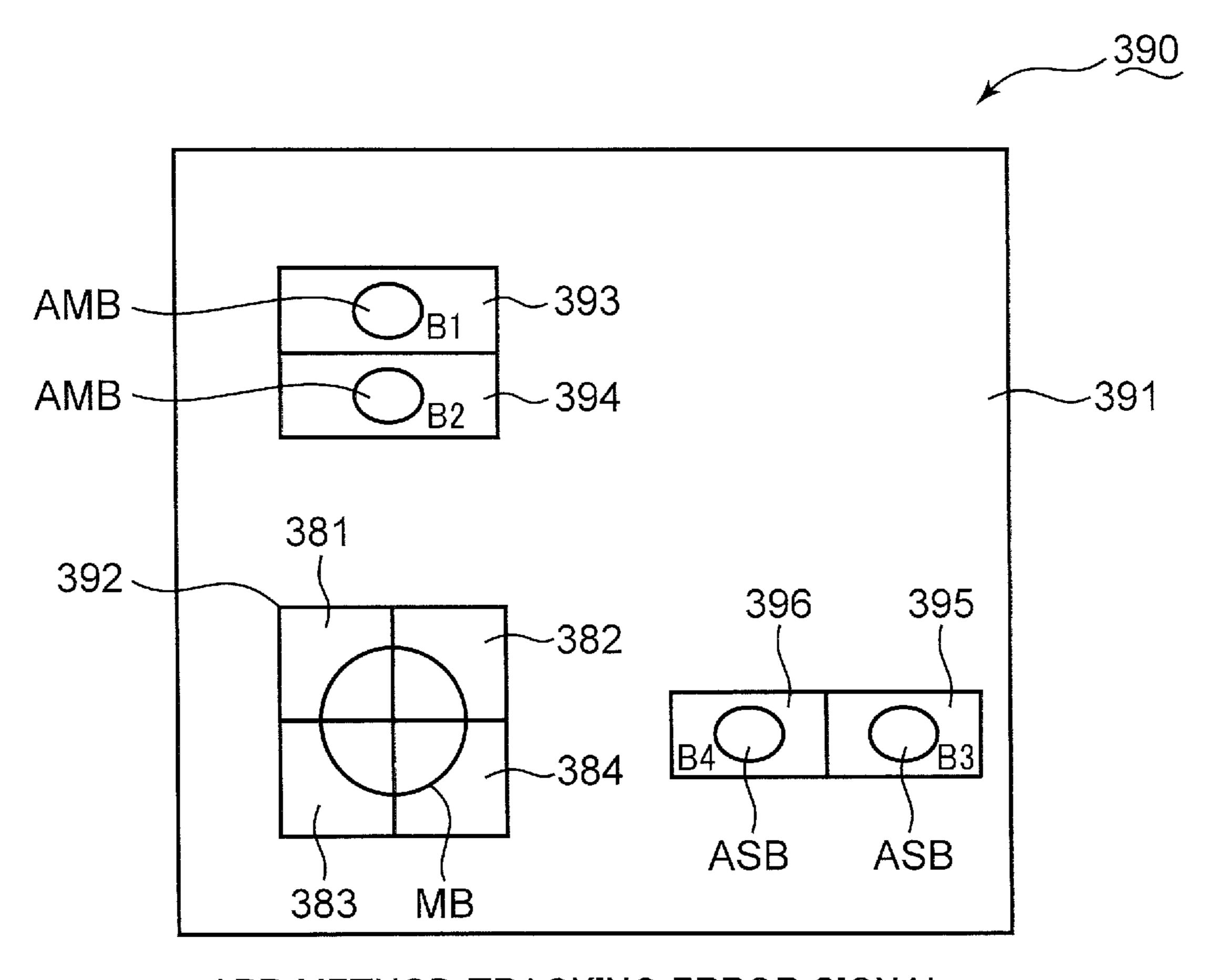
APP METHOD TRACKING ERROR SIGNAL = (B1 - B2) - k (B3 - B4) k : CONSTANT (NORMALLY 0.5 TO 5)
