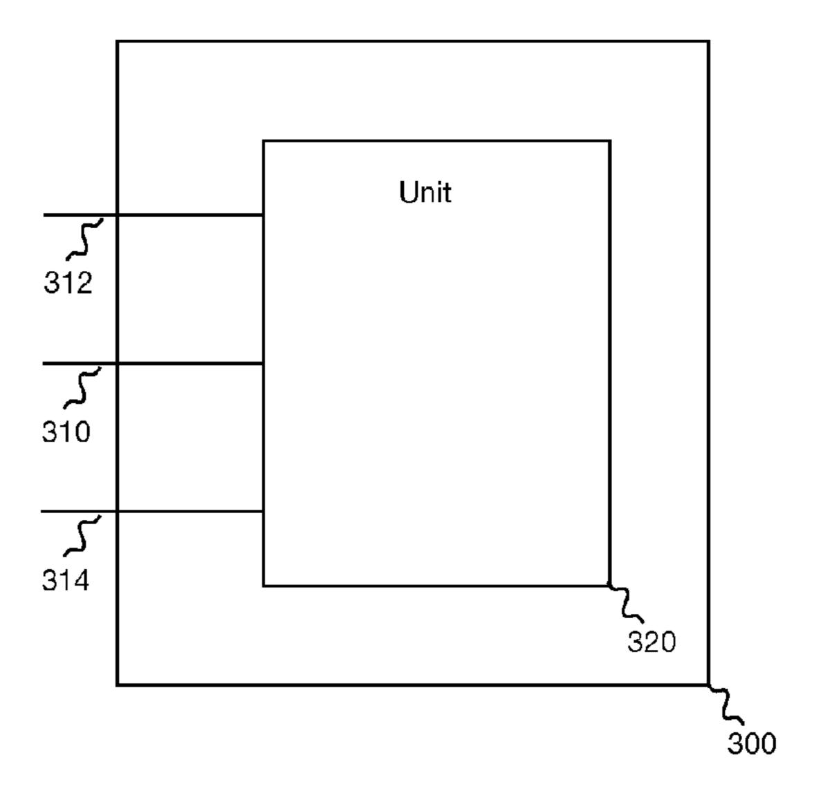
localization device 300 input for signal comprising information on a state of movement 310 input for receiving signals comprising information indicating rotational frequencies 312 input for receiving signals comprising information indicating a tire parameter 314 unit to assign to each of the plurality of wheels one location 320
