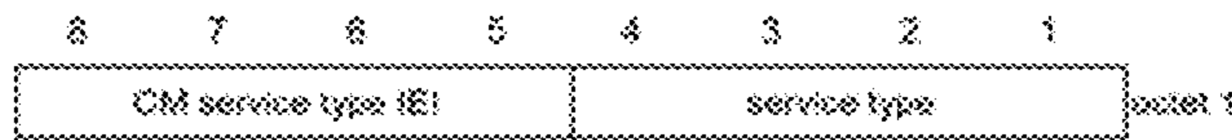
Figure 10.5.77/3GPP TS 24.008 CM Service Type information element
