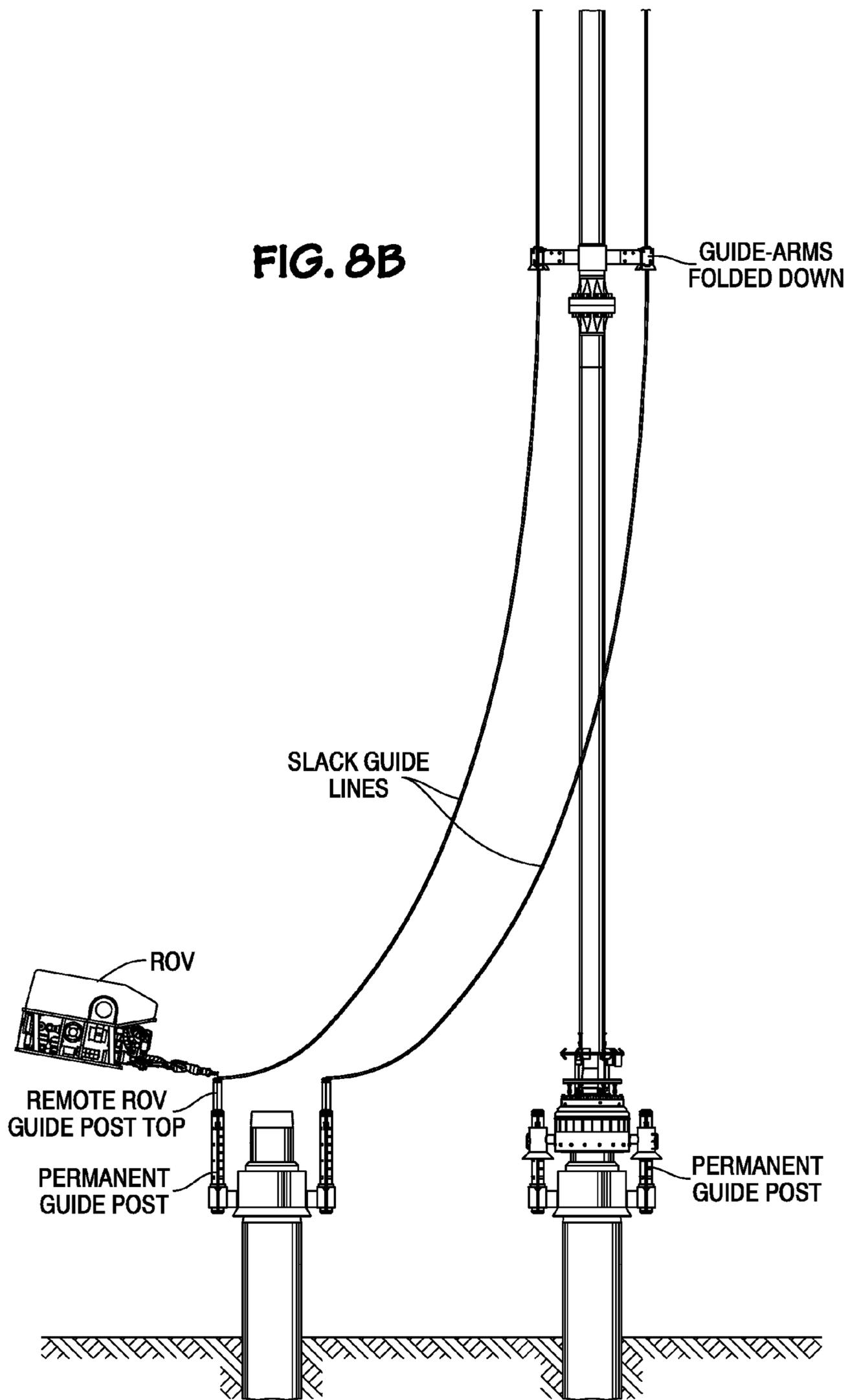
**STEP 2: ROV REMOVES AND RECONNECTS REMOTE POST TOPS.
