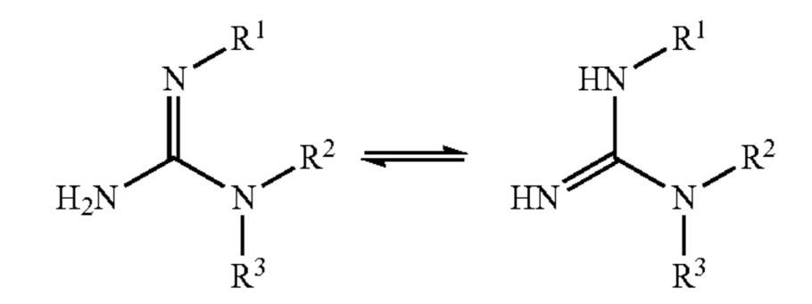
having the stated meanings for the residues R<sup>1</sup>, R<sup>2</sup> and R<sup>3</sup> as accelerators for cold-curing epoxy resin compositions. The curing of cold-curing epoxy resin systems may advantageously be accelerated with the assistance of these compounds.
