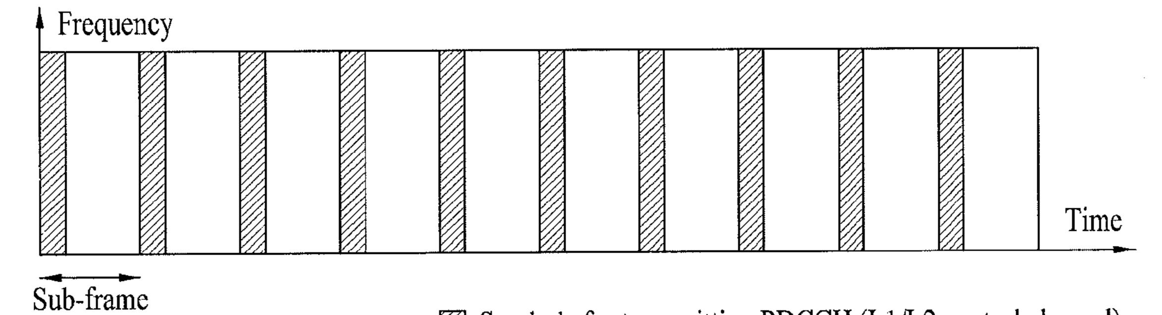
Symbols for transmitting PDCCH (L1/L2 control channel)
