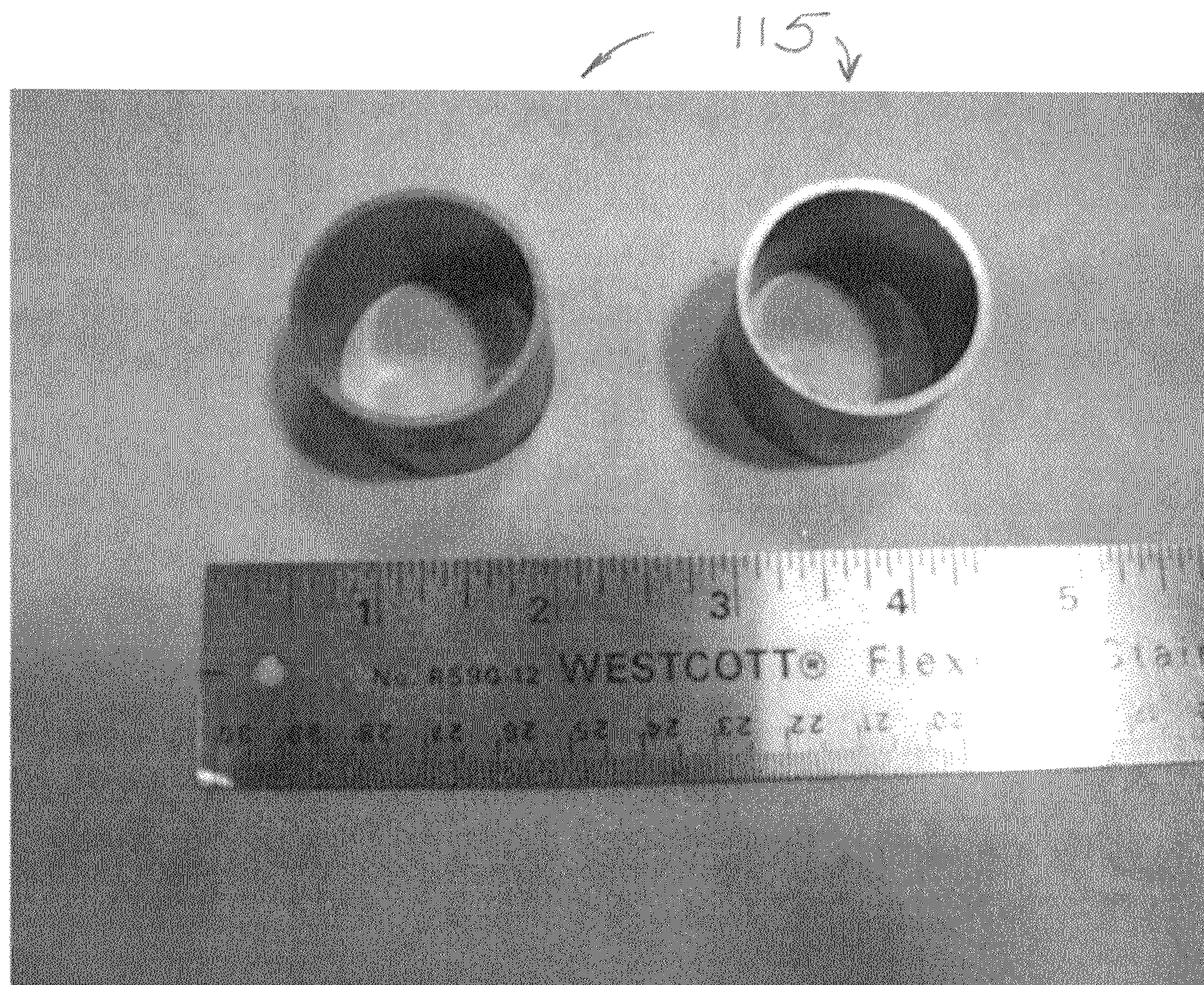
Figure 27. Top View of the Successfully CDC high pressure compacted Bonded Neo Thin Walled Ring Sample with Higher As-Pressed Green Densities without any Cracking after compacting at ~140-150 tsi After the Parts Removed from the Core Rod
