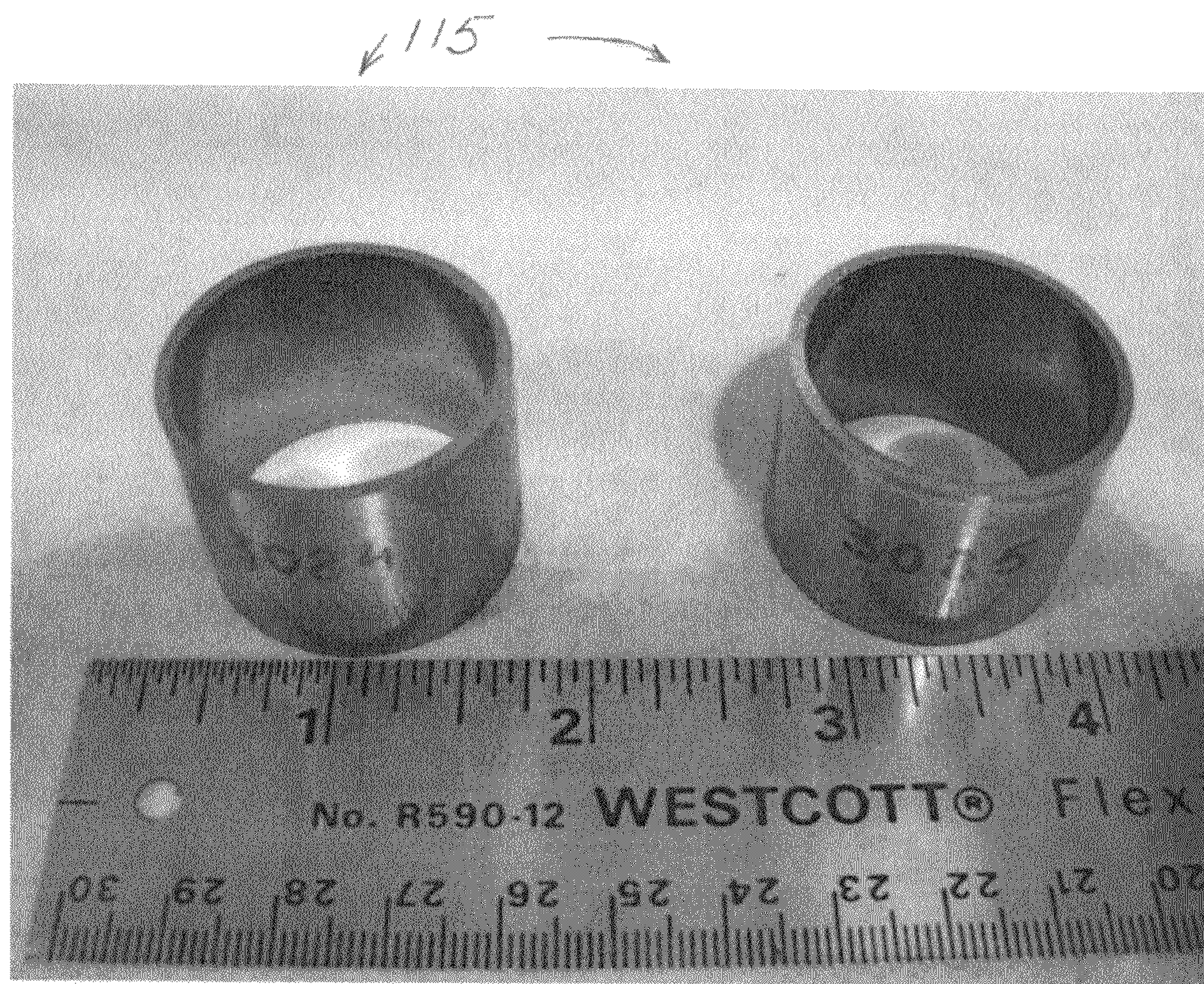
Figure 26. Angular Side views of the Successfully CDC high pressure compacted Bonded Neo Thin Walled Ring Sample with Higher As-Pressed Green Densities without any Cracking after compacting at ~140-150 tsi After the Parts Removed from the Core Rod.
