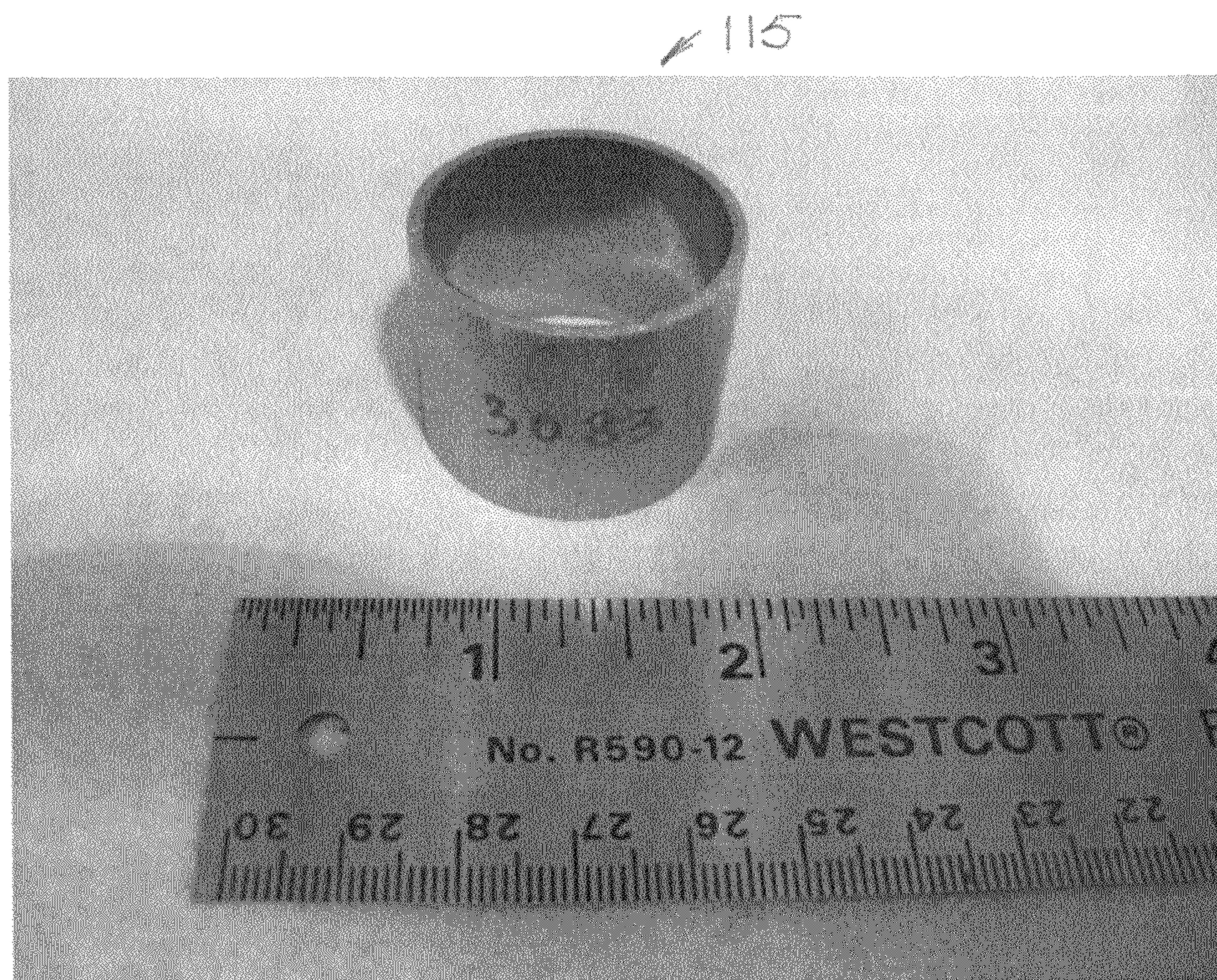
Figure 25. View of the CDC high pressure compacted Bonded Neo Thin Walled Ring at 95 tsi After the Part Removal from the Core Rod.
