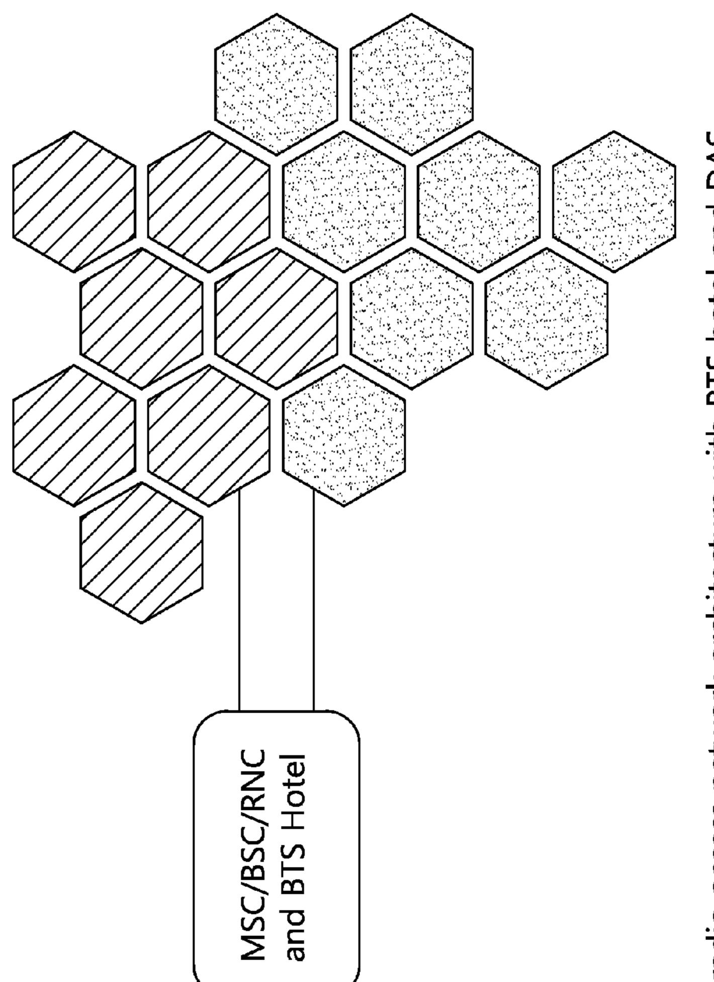
radio access network architecture with BTS hotel and DAS (each hexagon indicates cell)
