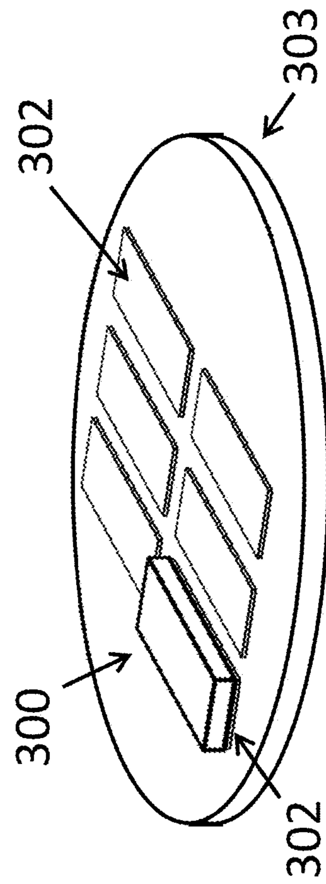
Figure 3: bond pads for alignment
