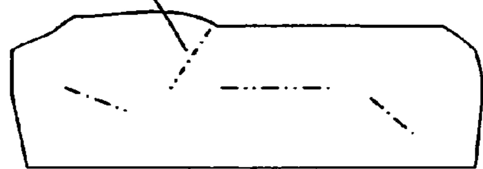
Graphene poly-crystal with incomplete grain boundaries (top view) (essentially a graphene single crystal with defects)
