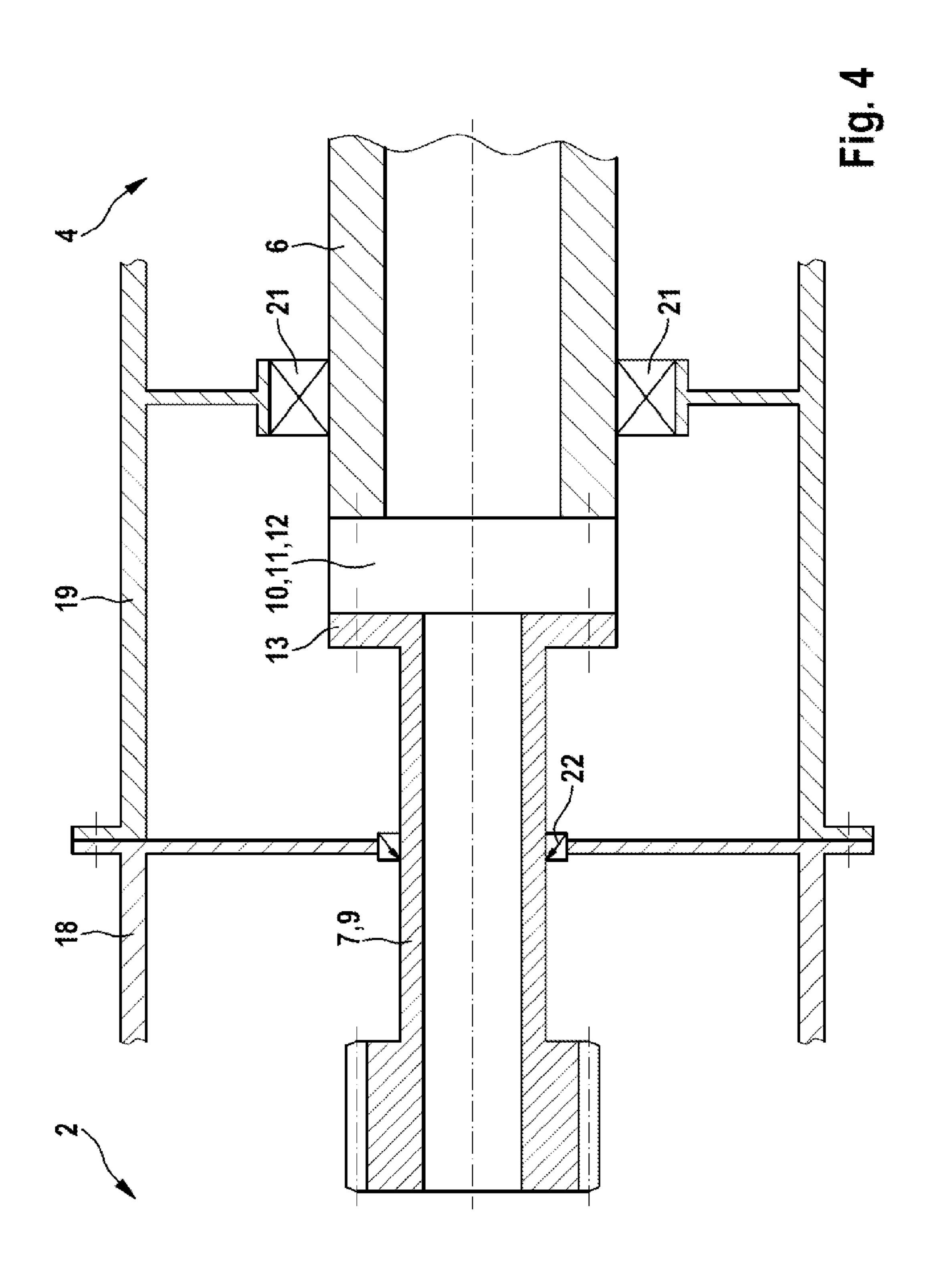
WIND POWER PLANT, HAVING COUPLING MEANS ARRANGED BETWEEN THE PLANETARY TRANSMISSION AND THE GENERATOR FOR THE PURPOSE OF COMPENSATING AXIAL, RADIAL AND ANGULAR MISALIGNMENT
