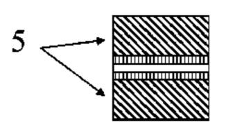
Growing group III nitride crystal on both sides of the wafer including the original seed crystal
