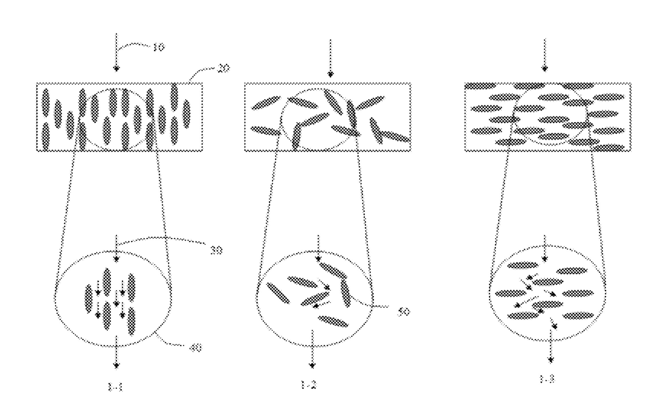
Figure 2: Determination of Orientation Of Nanoclay Platelets Using SAXS
