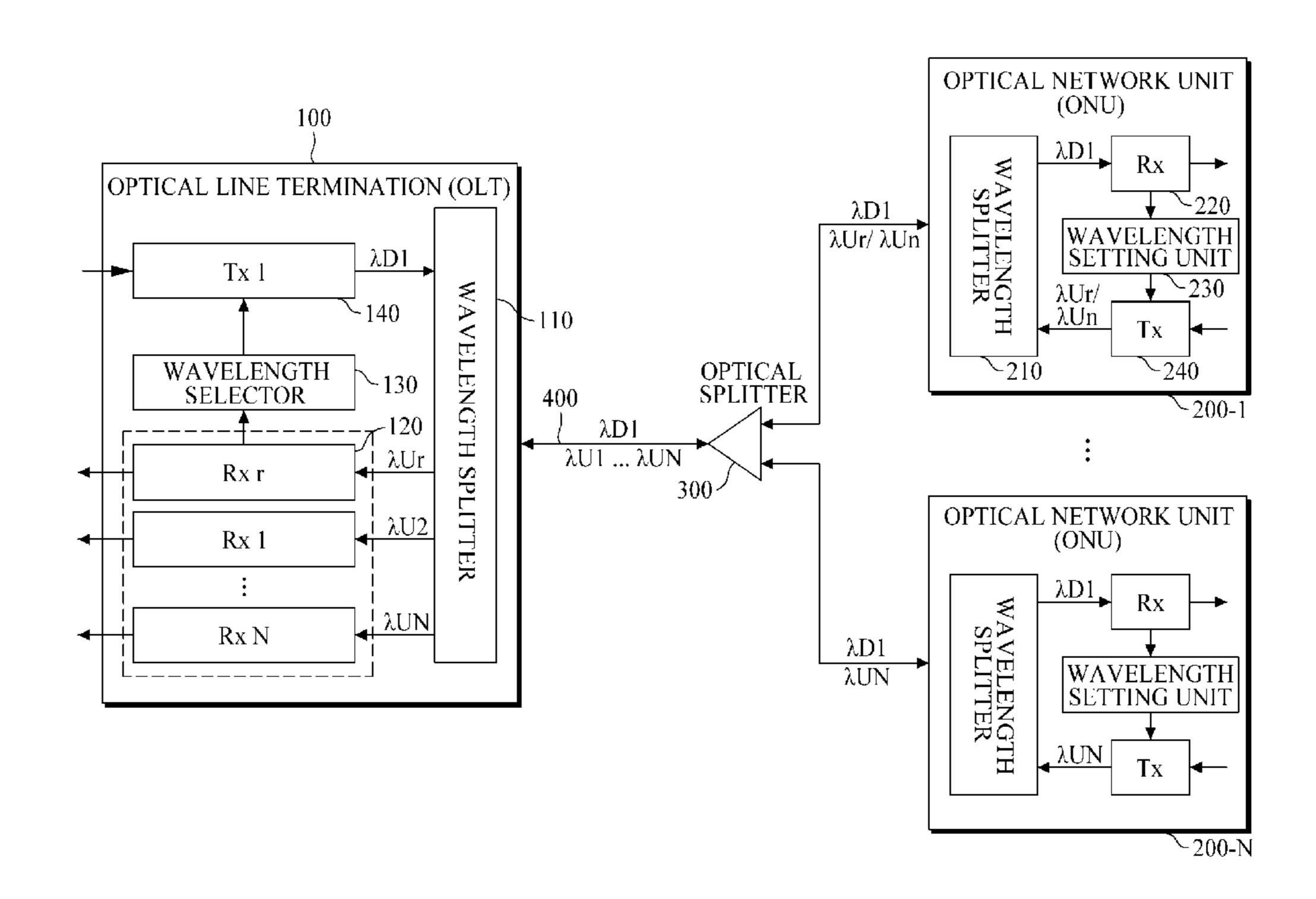
WORK UNIT U) WAVELENGTH SPLITTER WAVELENGTH SPLITTER WAVELENGTH SPLITTER 130
