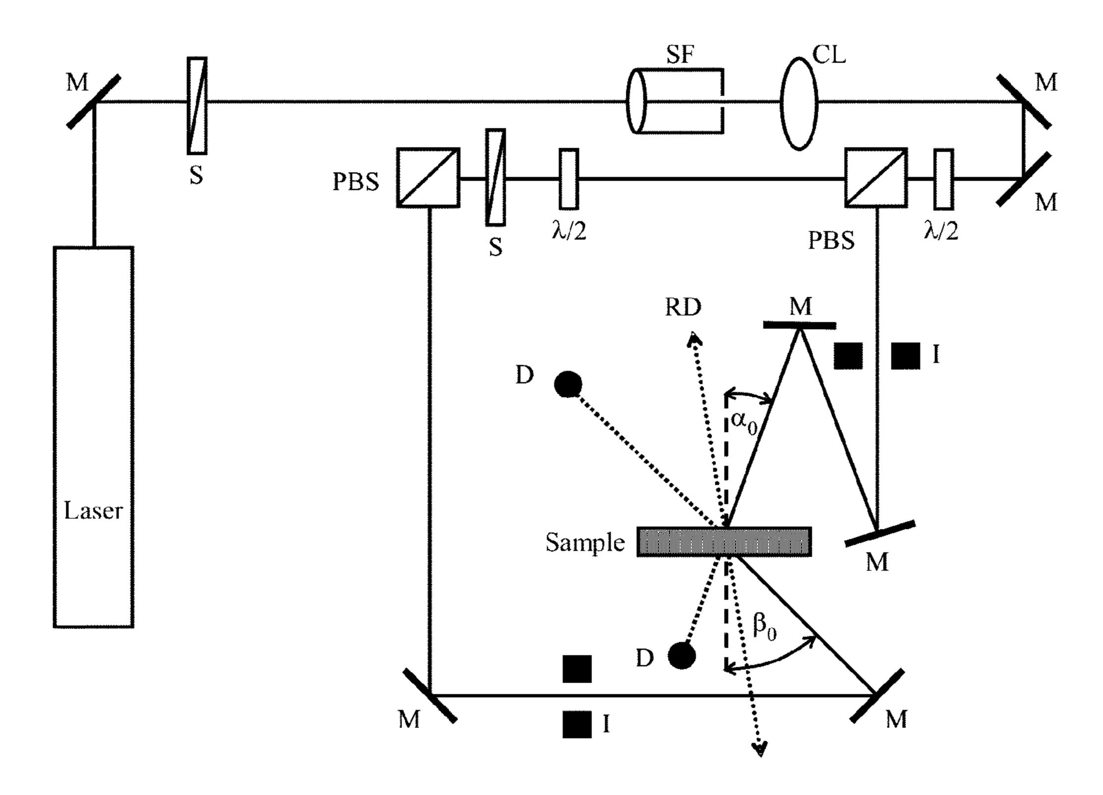
Figure 1 shows the geometry of a holographic media tester (HMT) at  $\lambda = 633$  nm (He-Ne laser): M = mirror, S = shutter, SF = spatial filter, CL = collimator lens,  $\lambda/2 = \lambda/2$  plate, PBS = polarisation-sensitive beam splitter, D = detector, I = iris diaphragm,  $\alpha_0 = -21.8^{\circ}$ ,  $\beta_0 = 41.8^{\circ}$  are the angles of incidence of the coherent beams measured outside the sample (outside the medium). RD = reference direction of the turntable.
