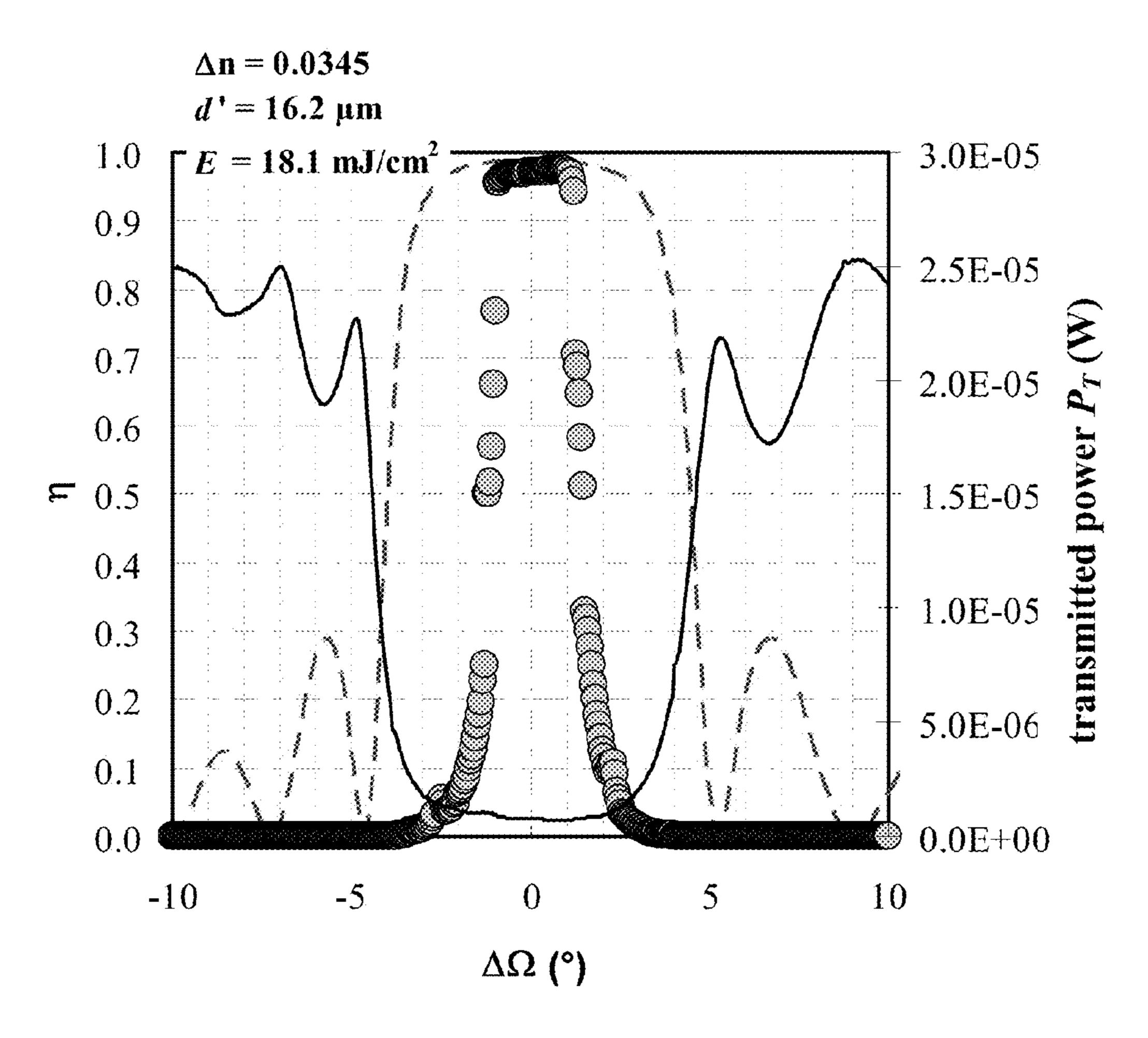
Figure 2 shows the measured transmitted power  $P_T$  (right y-axis) as a solid line plotted against the angle detuning  $\Delta\Omega$ , the measured diffraction efficiency  $\eta$  (left y-axis) as solid circles plotted against the angle detuning  $\Delta\Omega$  (in so far as permitted by the finite size of the detector), and the adaptation of the Kogelnik theory as a broken line (left y-axis).
