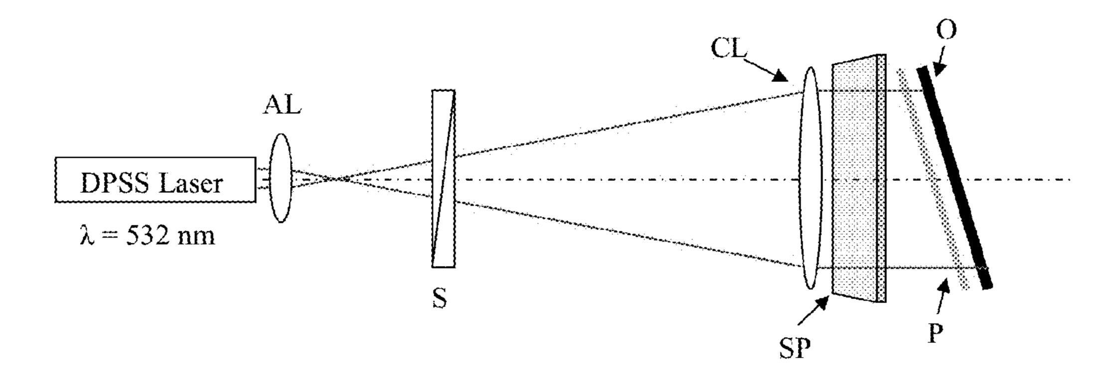
Figure 3 shows the measuring arrangement for testing the holographic properties for wavelengths of 635 and 532 nm.
