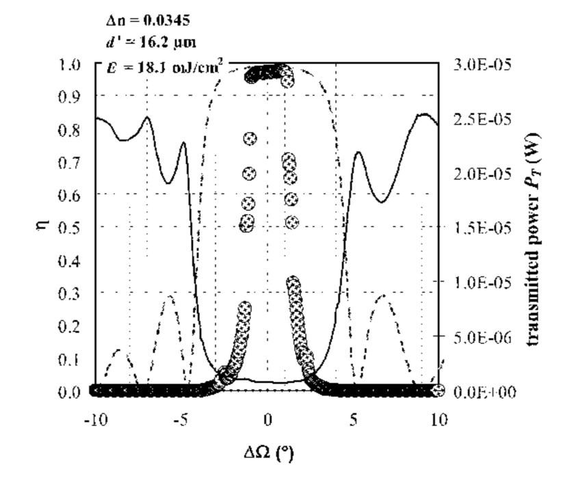
shows the measured transmitted power  $P_{\tau}$  (right y-axis) as a solid line plotted against the angle detuning  $\Delta\Omega$ , the measured diffraction efficiency  $\eta$  (left y-axis) as solid circles plotted against the angle detuning  $\Delta\Omega$  (in so far as permitted by the finite size of the detector), and the adaptation of the Kogelnik theory as a broken line (left y-axis).
