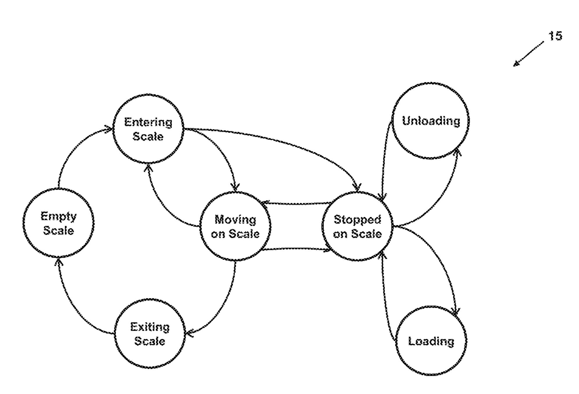
Note: Gross weight < threshold resets from any state to Empty Scale
