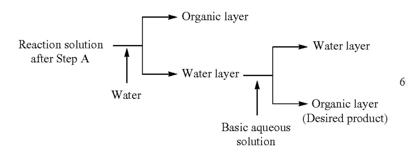
In Step B of the present invention, firstly water is added to, and mixed with the reaction solution, and then the water layer
