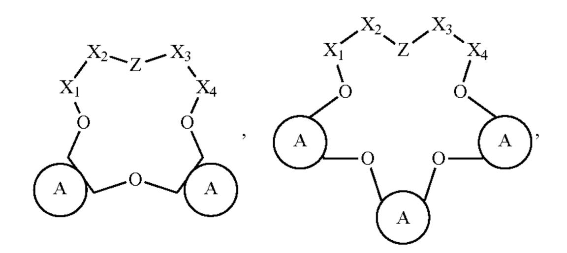
wherein, at each occurrence, A independently comprises a carbocyclic ring or —CH<sub>2</sub>CH<sub>2</sub>—;
