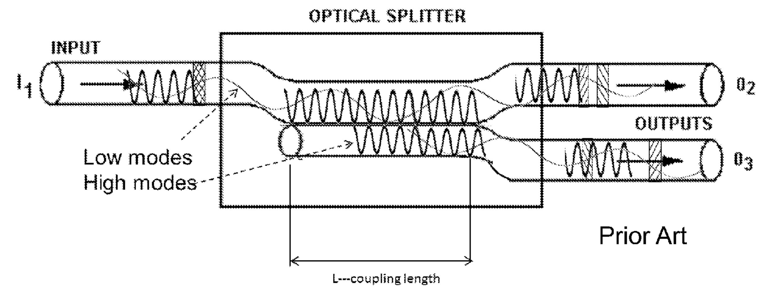
With non-symmetry splitting ratio mode dispersion between high modes & low modes at high speed is even larger (10Gbps above)
