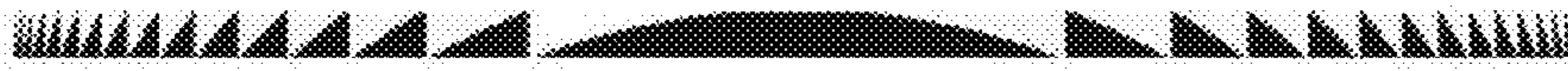
Phase Wrapping Convex Lens 1201
