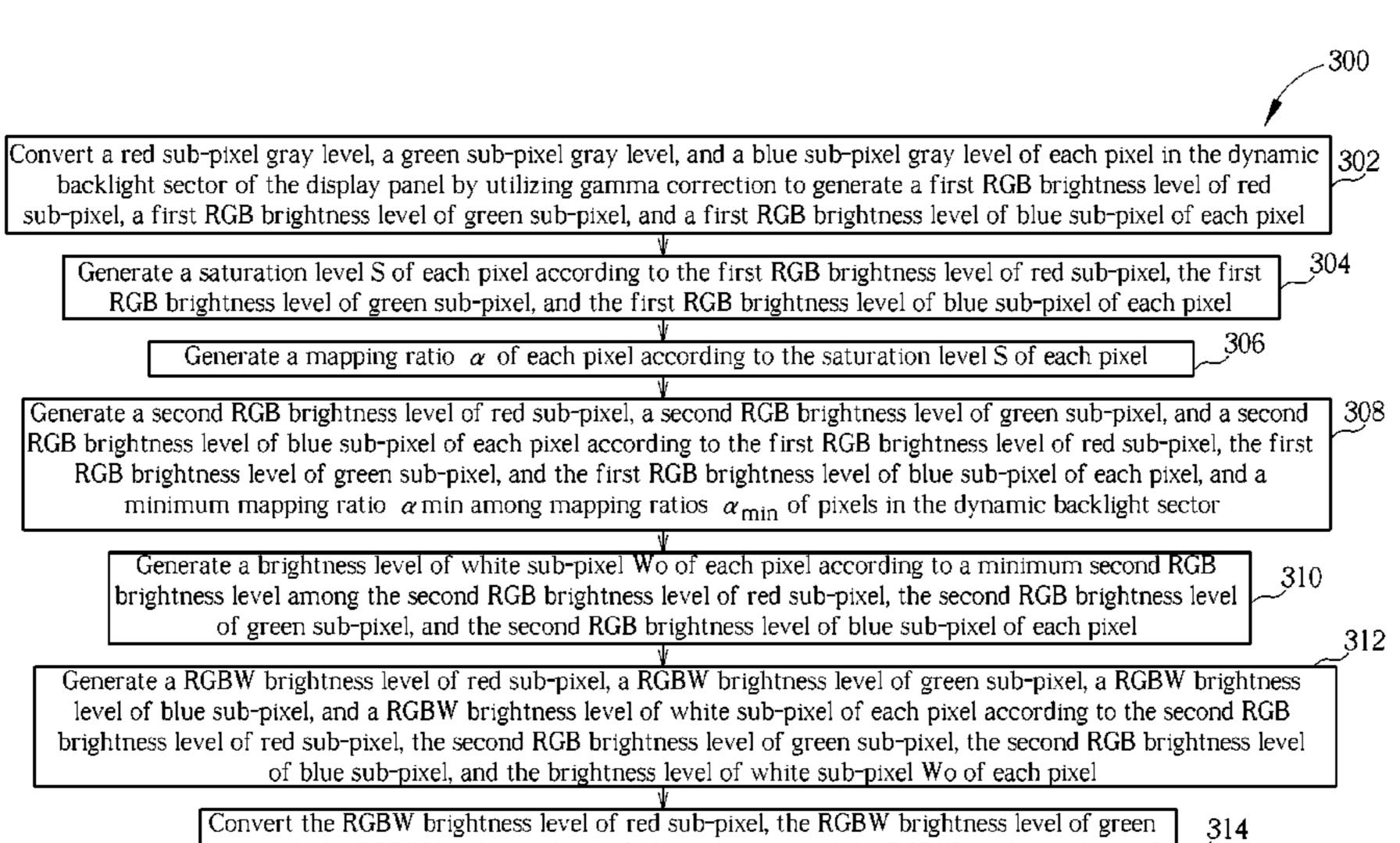
Convert the RGBW brightness level of red sub-pixel, the RGBW brightness level of green sub-pixel, the RGBW brightness level of blue sub-pixel, and the RGBW brightness level of white sub-pixel of each pixel by utilizing inverse gamma correction to generate a RGBW gray level of red sub-pixel, a RGBW gray level of green sub-pixel, a RGBW gray level of blue sub-pixel, and a RGBW gray level of white sub-pixel of each pixel
