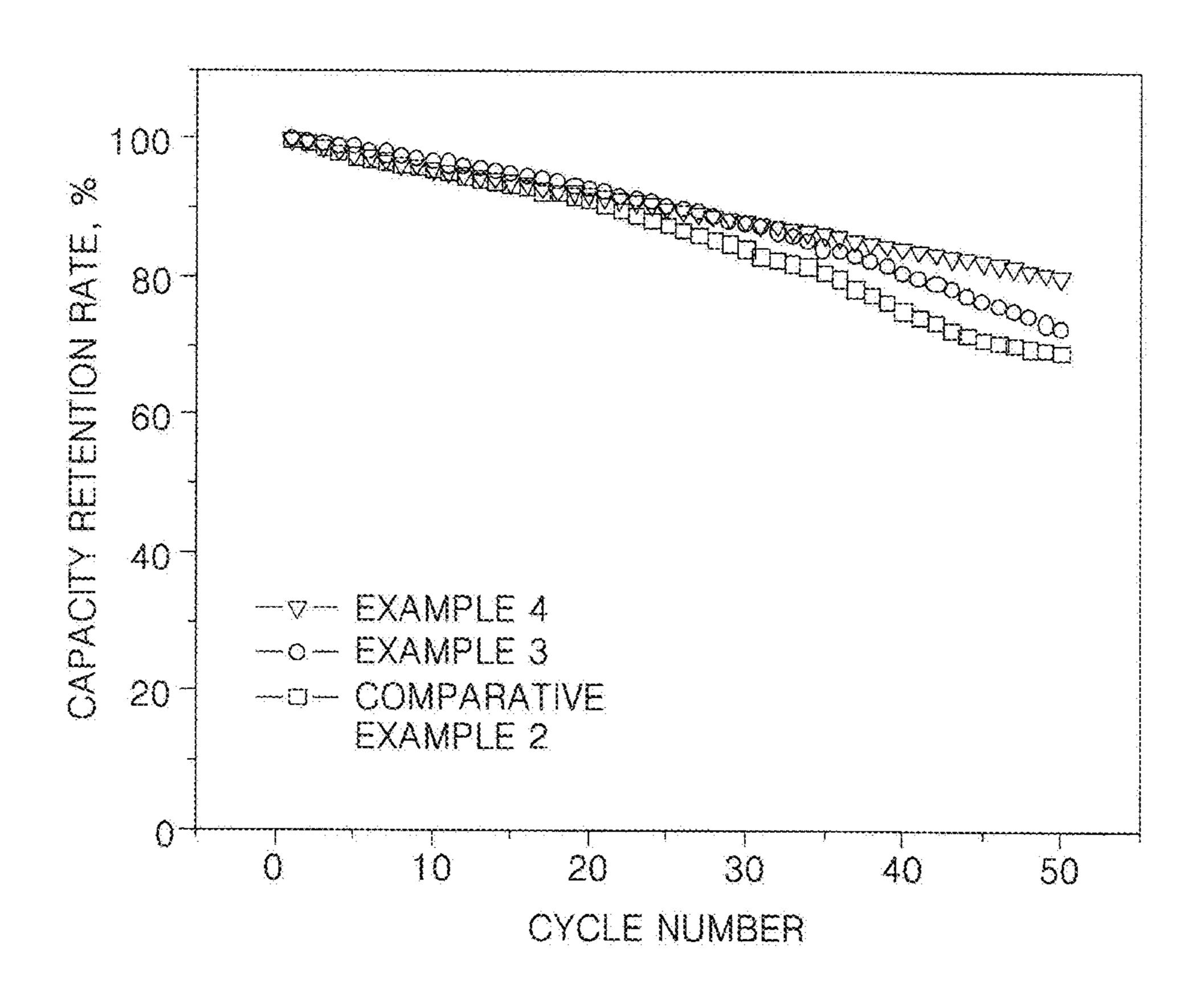
NEGATIVE ACTIVE MATERIAL FOR LITHIUM BATTERY, METHOD OF PREPARING THE NEGATIVE ACTIVE MATERIAL, AND LITHIUM BATTERY EMPLOYING THE NEGATIVE ACTIVE MATERIAL
