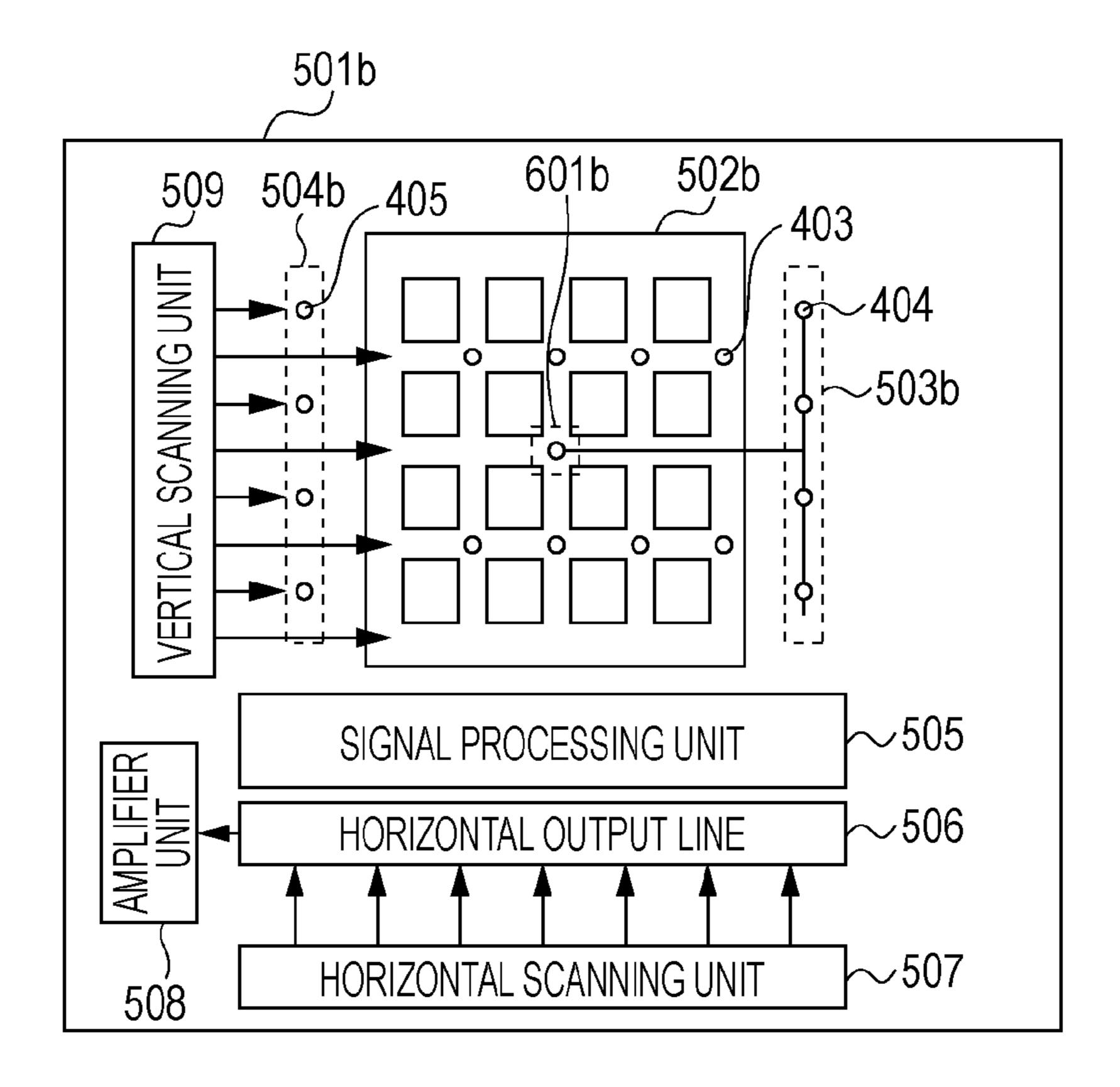
SOLID-STATE IMAGE PICKUP DEVICE HAVING REFERENCE VOLTAGE SUPPLY LINE ON A FIRST SUBSTRATE AND POWER SUPPLY LINES TO SUPPLY VOLTAGES TO THE REFERENCE VOLTAGE SUPPLY LINE ON A SECOND SUBSTRATE
