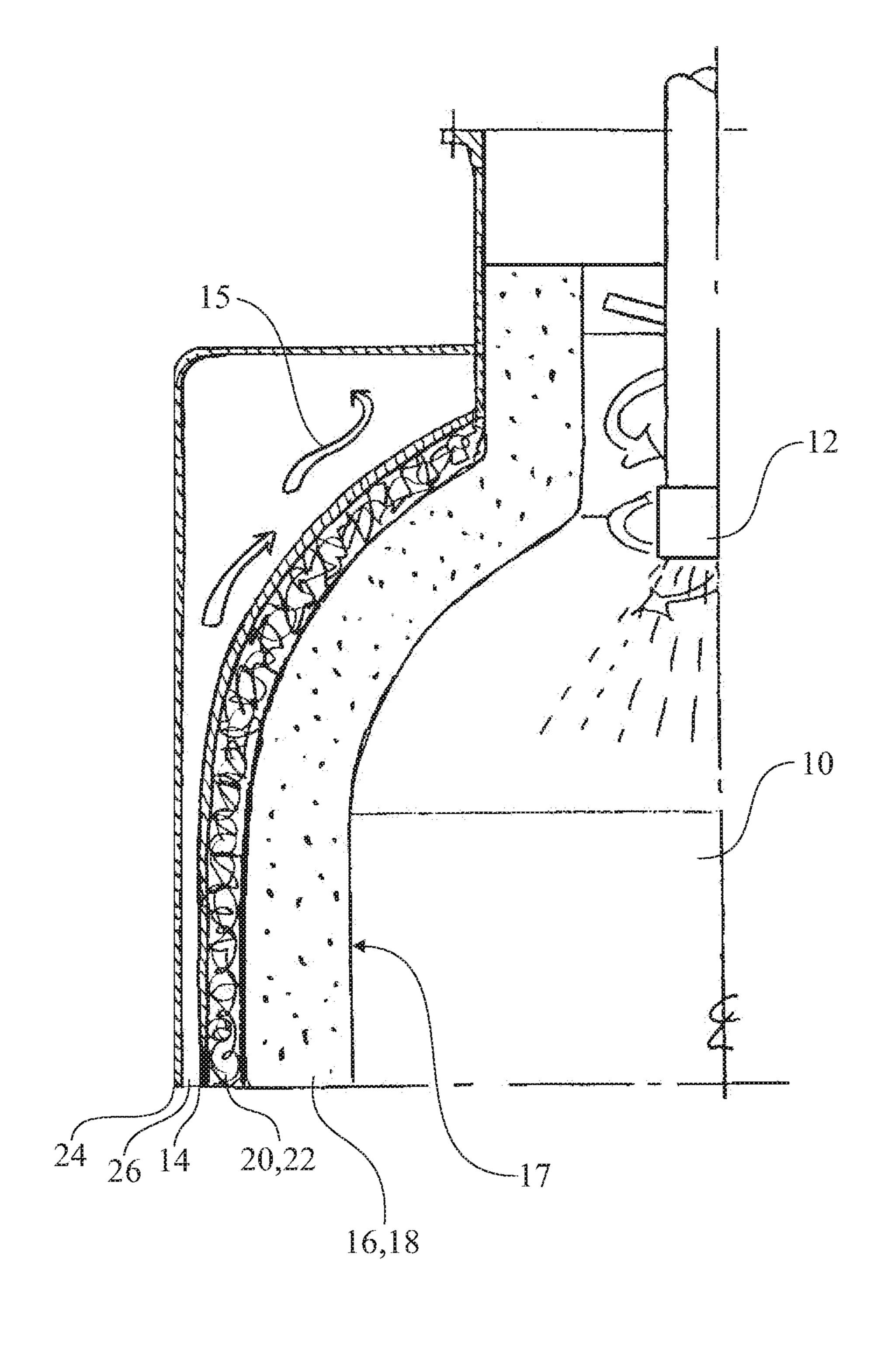
METHOD FOR ARRANGING A CHEMICAL BARRIER IN A GASIFYING REACTOR FOR BLACK LIQUOR, A CHEMICAL GASIFYING REACTOR, A BARRIER LAYER OF A REACTOR AND A METHOD FOR MANUFACTURING A BUILDING BLOCK FOR SUCH A BARRIER LAYER
