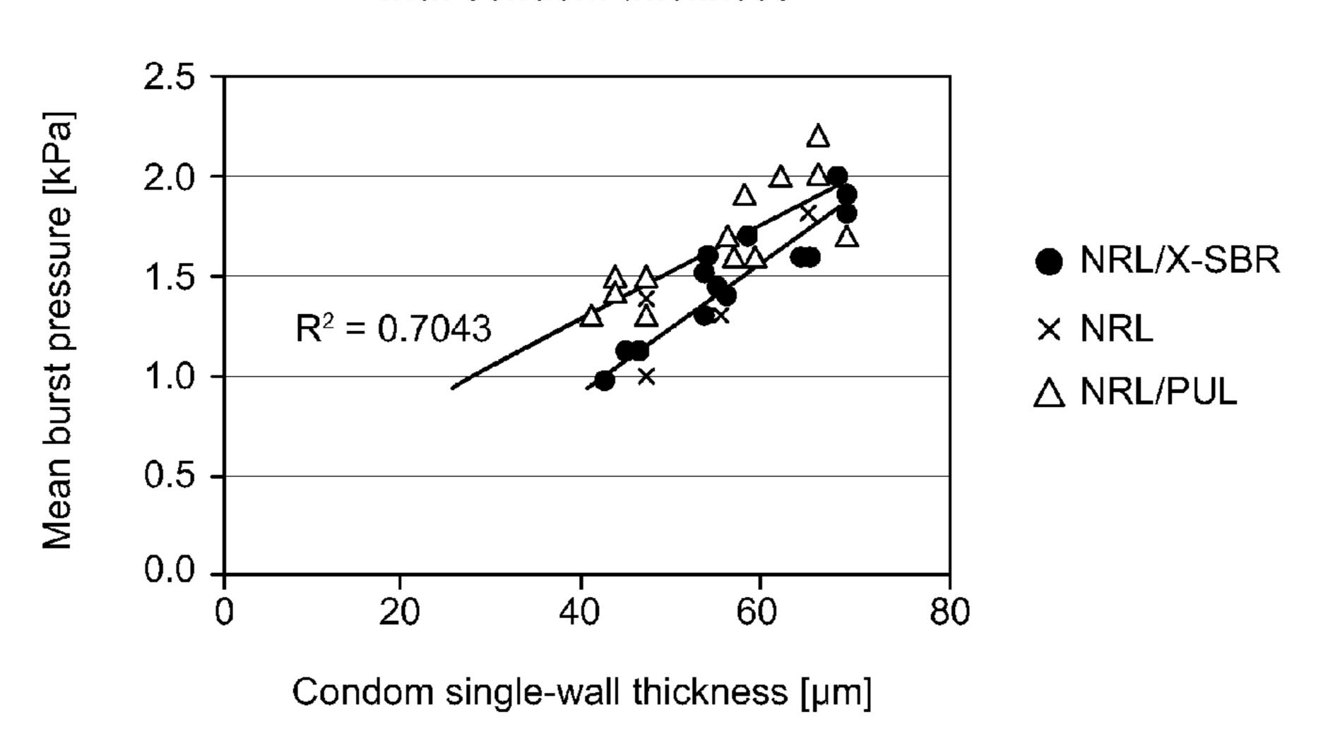
The data are taken from Figure 1 (NRL/X-SBR), Figure 2 (NRL) and Figure 3 (NRL/PUL) The least square fits for the NRL and NRL/X-SBR data overlap and only begin to diverge at low thickness/burst pressure values
