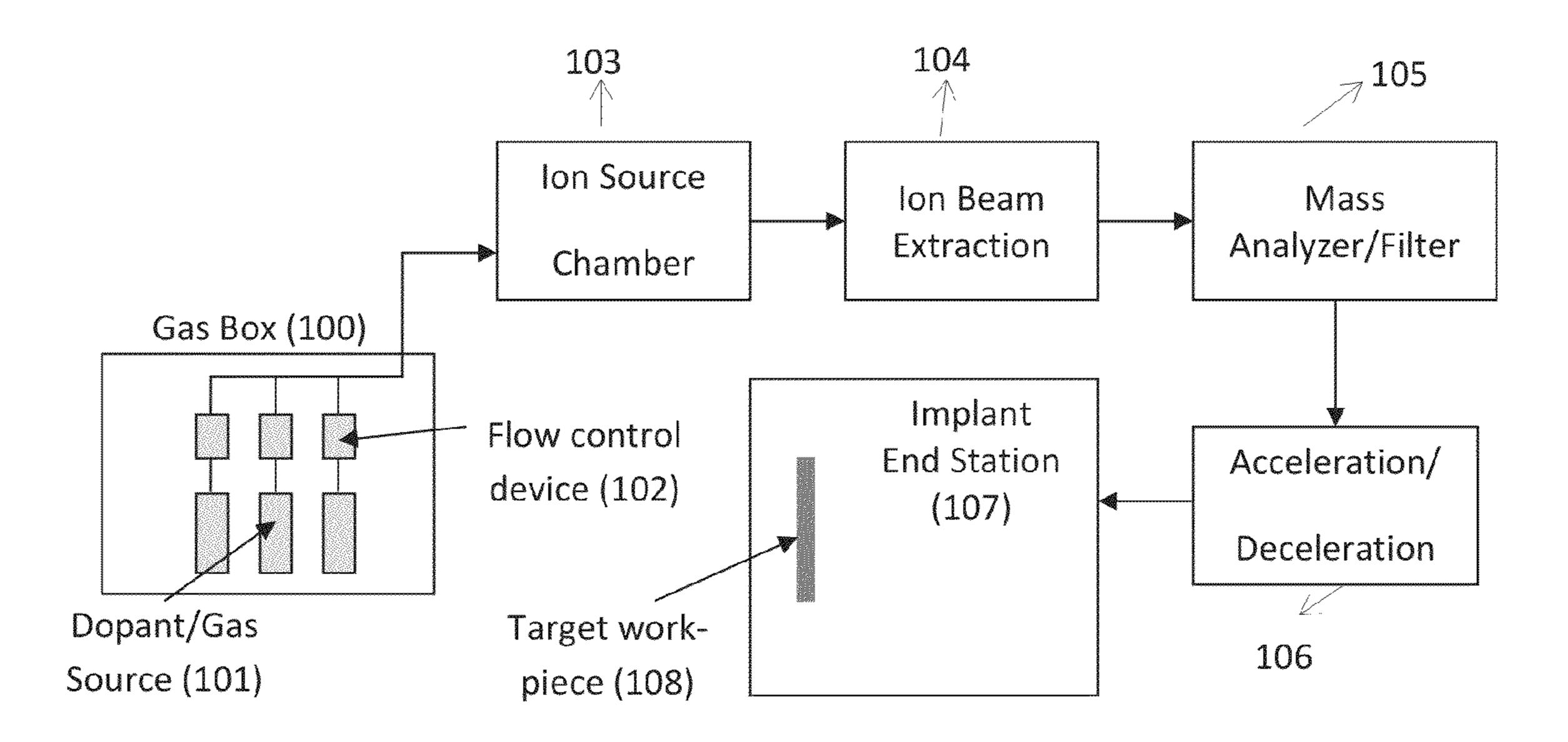
Schematic of beamline ion implant system
