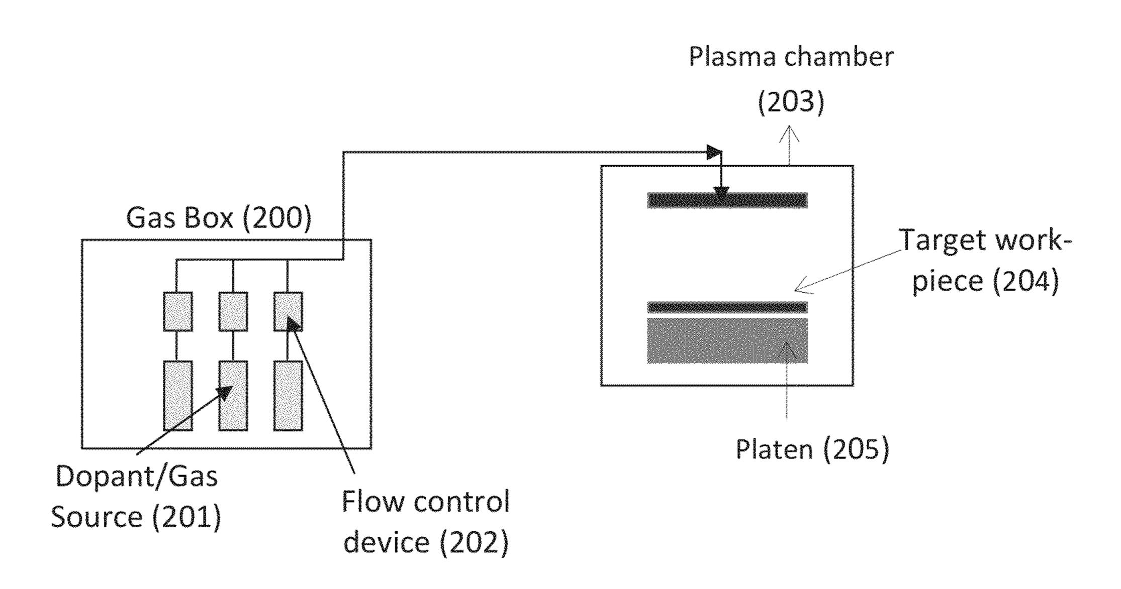
Schematic of plasma immersion ion implant system
