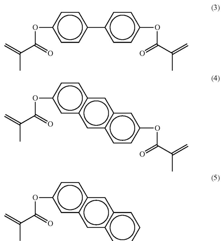
For production of the liquid crystal cell described in Example 1, compounds represented by the above chemical formulae (4) and (5) to be used as monomers for forming a PSA layer were synthesized. Meanwhile, the synthesis method of the compounds is not limited to the method below.
